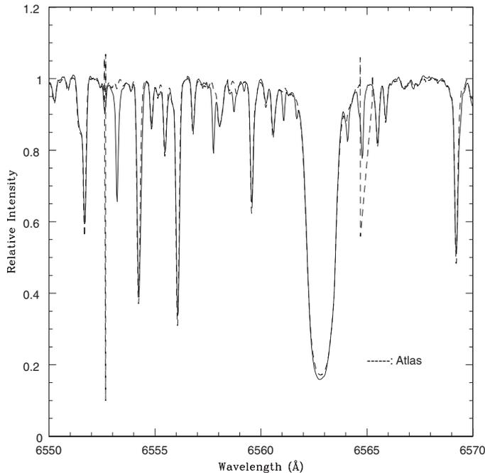
**Figure 2.** Spectrum of Arcturus obtained with fiber fed echelle spectrometer at VBT superposed on Kit Peak Atlas spectrum.
