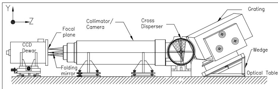
**Figure 1.** Opto-mechanical layout of the spectrometer. F/5 beam emerging from the slit is fed into the collimator by a folding mirror. The collimated beam then passes through the cross disperser (prism) and gets pre-dispersed and illuminates the echelle grating. The dispersed beam from the grating again passes through the prism a second time and finally comes to focus on the CCD plane where the spectrum is recorded.
