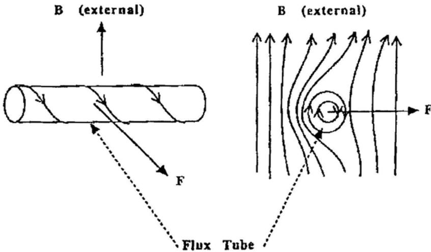
**Figure 2.** A horizontal flux rope in vertical external fields experiences a force  $F$  that is repulsive on one side and attractive on the other.
