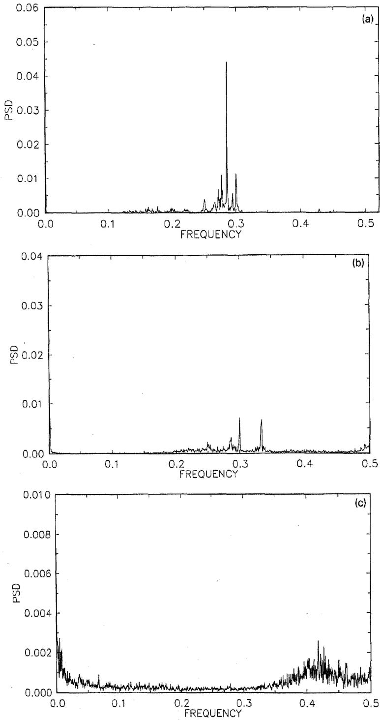
**Figure 1(a-c).** Power spectra for the system (1), with  $\cos(Y_n)$  used as the variable, calculated with  $X_0=0.5$ ,  $Y_0 = 0.505$  and at different values of  $k$ : (a)  $k = 0.99$ , (b)  $k = 1.50$ , (c)  $k = 2.99$ .
