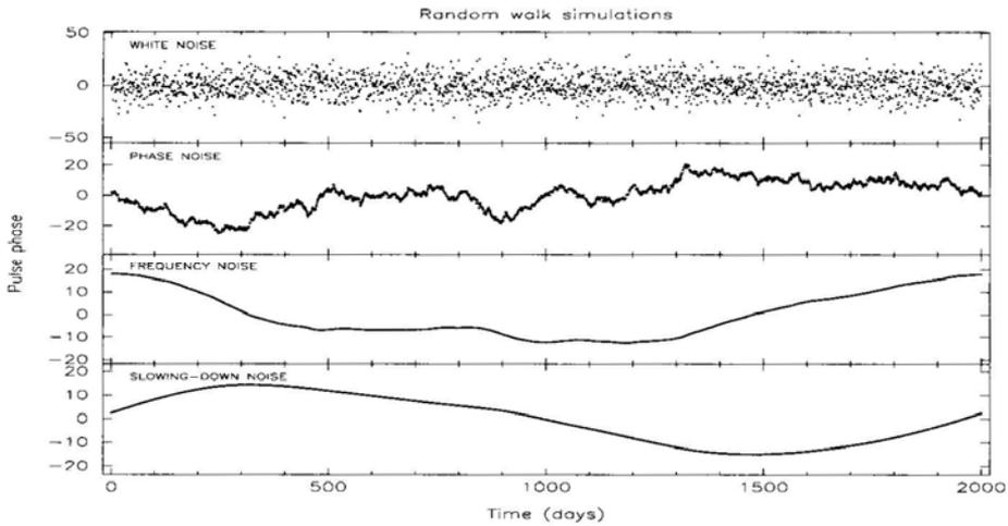
**Figure 1.** Uniformly sampled time sequences which simulate white noise (WN), phase noise (PN), frequency noise (FN) and slowingdown noise (SN) respectively, with 0.1% of white noise added to the sequences for PN, FN and SN.
