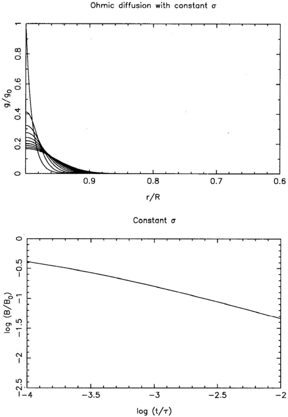
Figure 4: Ohmic diffusion of crustal magnetic field, assuming a constant electrical conductivity in the crust. The upper panel shows the evolution of the  $g$ -profile and the bottom panel the evolution of the field strength at the surface. See text for details.
