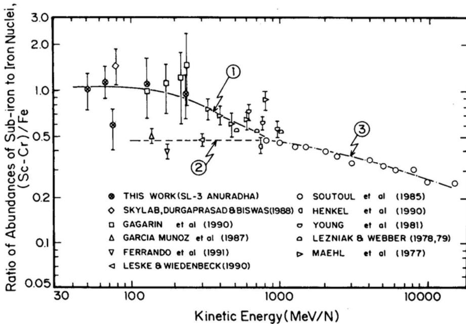
**Figure 2.** The ratio of abundances of (Sc-Cr) to Fe ions vs kinetic energy in 30 MeV/N to  $\sim 10$  GeV/N. The eye fit line denoted by 1 represents approximate curve for the ratio measured inside the magnetosphere in Skylab, Spacelab-3 and Soyuz-6, whereas the eye fit line 2 shows the value of the ratio measured in the interplanetary space. The line 3 shows the variation of the ratio in the high energy region in 1-10 GeV/N measured in HEAO-3 spacecraft.
