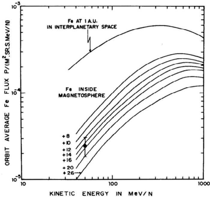
**Figure 3.** Fe-flux vs 1 AU outside the magnetosphere is shown in the uppermost curve, and the calculated orbit average Fe fluxes inside the magnetosphere are shown by the lower set of curves for assumed mean ionization states of  $\text{Fe}^{+8}$  to  $\text{Fe}^{+26}$ . The measured orbit average flux in SL-3 at 50 MeV/N is shown which indicates that the ionization state of these Fe particles is +15.
