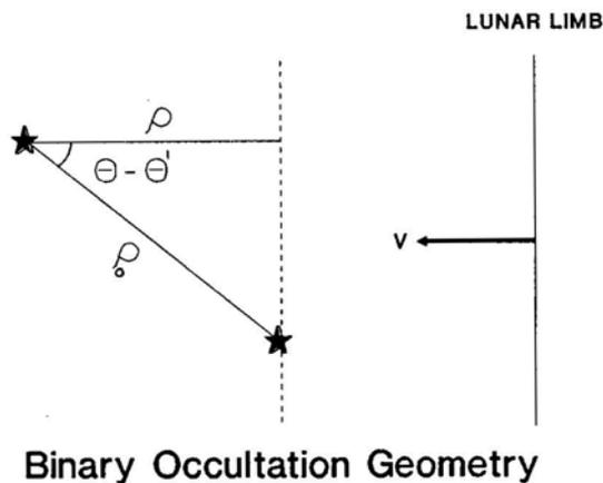
**Figure 3.** A simplified picture of a binary occultation.  $V$  is the velocity component of the moon perpendicular to the limb at the position angle ( $\theta'$ ) of occultation assumed the same for both components of the binary. Position angle of the binary system is denoted by  $\theta$ .  $\theta$  and  $\theta'$  are measured from celestial North through East.
