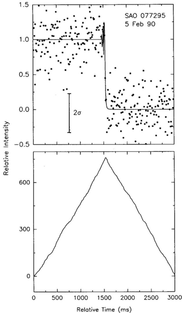
**Figure 4a.** Occultation data along with the integral curve are given for the observations of SAO 077295 ( $m_v = 6.5$ , K2). The source is not a binary as can be seen from the triangular shape of the integral curve. The main source of noise in the data is the sky photon noise due to the bright sky near the moon.  $2\sigma$  error bar corresponding to this noise is shown.
