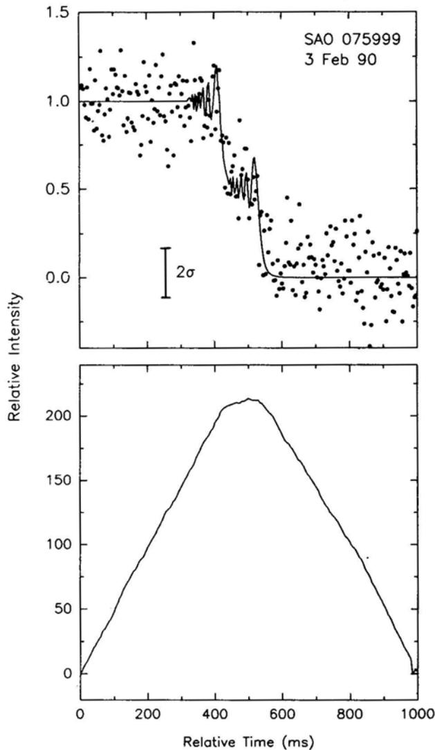
**Figure 4b.** Binary occultation of SAO 075999 ( $m_v = 5.9$ , A3 V) observed on 3 Feb 1990 in the B filter. The component stars are of equal brightness and are seen clearly separated by 108 milliseconds corresponding to 55 milliarcsec. A composite point source diffraction pattern is fitted to the data.
