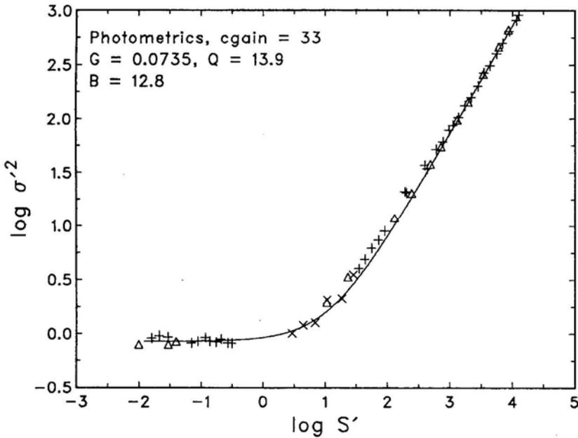
**Figure 2.** The logarithmic plot of variance versus signal together with the theoretical fit for the Photometrics CCD system and  $cgain = 33$  based on the data obtained in 1992 January. The fit is based on spectroscopic data in the range  $300 \leq S \leq 10000$ , and the bias statistics. Other details are as in Fig. 1. Surprisingly, data from a different set ( $\times$ ) obtained on 1991 May 12, agrees with the theoretical fit even at low signal values.
