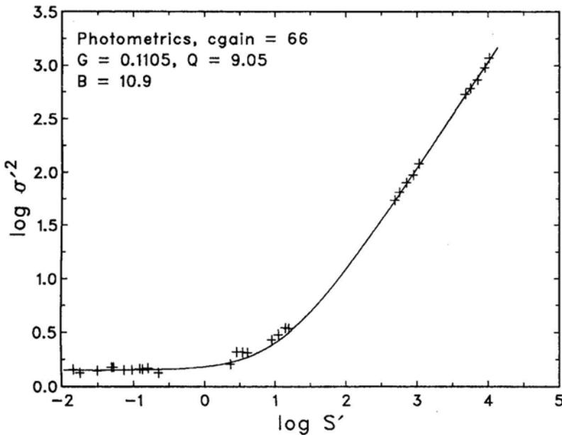
**Figure 3.** The logarithmic plot of variance versus signal together with the theoretical fit for the Photometrics CCD system and  $cgain = 66$ . The fit is based on data in the range  $S > 500$ , and the bias statistics. Other details are as in Fig. 1.
