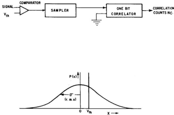
**Figure 9.** A schematic of the technique used to measure the power of a signal using a one-bit correlator and the threshold detector.
