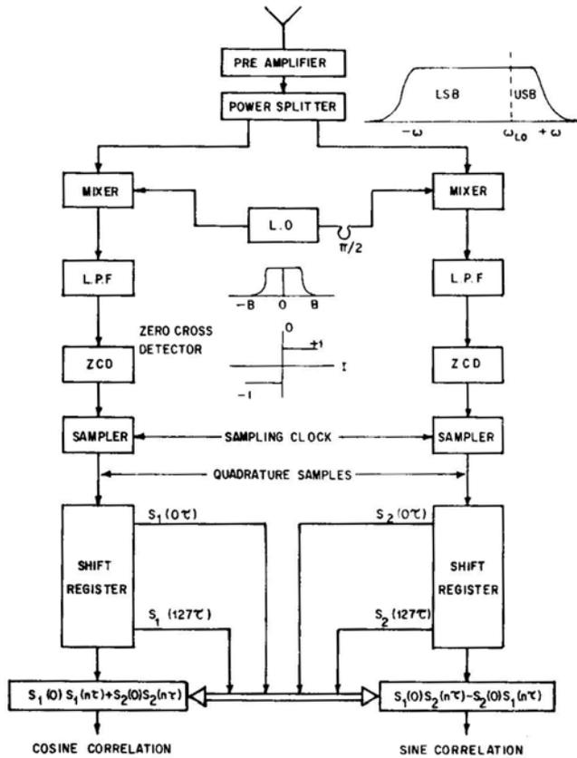
**Figure 6b.** The scheme for obtaining quadrature samples and correlation coefficients in the conventional DSB system, employed for spectral-line observations in the present receiver. Cosine transform of cos correlator output gives the sum of the two sidebands (USB +LSB). Sine transform of sine correlator output gives the difference between the two sidebands (USB — LSB).
