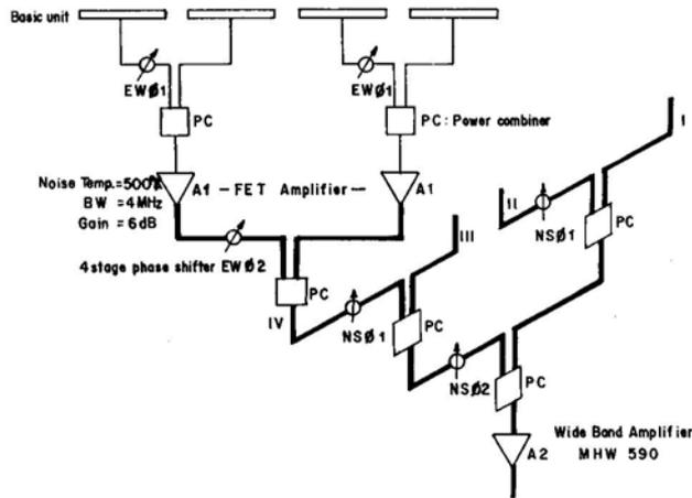
**Figure 3.** The Christmas-tree configuration of the EW array consisting of 4 basic units in each row is shown in detail.
