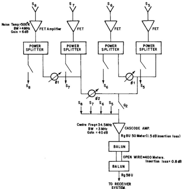
**Figure 4.** The configuration used in the S array for the sky survey.  $S_5, S_6, S_7, S_8$  refer to rows of basic units in the S array.
