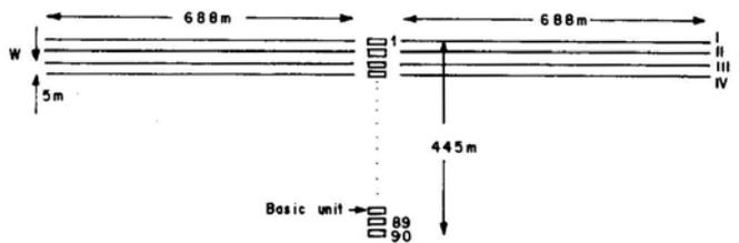
**Figure 1b.** The Gauribidanur radio telescope (GEETEE). Collecting area: EW array  $\approx 12,000 \text{ m}^2$ , S array  $\approx 7,000 \text{ m}^2$ , EW  $\times$  S in correlation mode  $\approx 18,000 \text{ m}^2$ .
