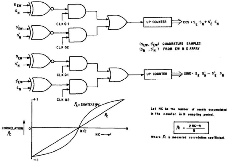
**Figure 8.** This figure illustrates a scheme for addition of correlations required for a DSB system. A DSB system needs four multipliers to obtain the desired correlation counts  $N_C$ . The equation and the graph describe the relation between the desired correlation coefficient  $\rho_A$  and  $N_C$ .
