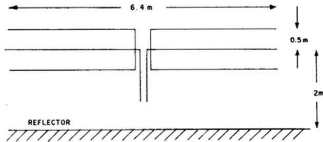
**Figure 1a.** Four fat dipoles (one of which is shown in this figure) are combined along the EW direction through open-wire transmission lines and appropriate impedance transformers to form a basic unit. Characteristic impedance of the dipole:  $600\Omega$ , Bandwidth: 25–35 MHz with a VSWR of 1.1–1.5, Polarization: linear, oriented along EW.
