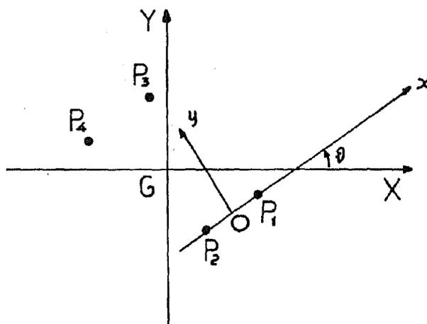
**Figure 1.** The inertial frame  $GXY$  and the rotating frame  $0xy$ .  $G$  is the mass centre of the system and  $0$  is the mass centre of  $P_1$  and  $P_2$ .
