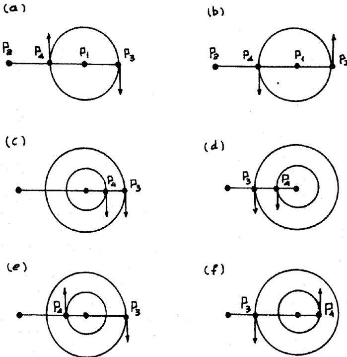
**Figure 3.** Periodic orbits in the case where  $P_3$  and  $P_4$  revolve around  $P_1$  (shown schematically).
