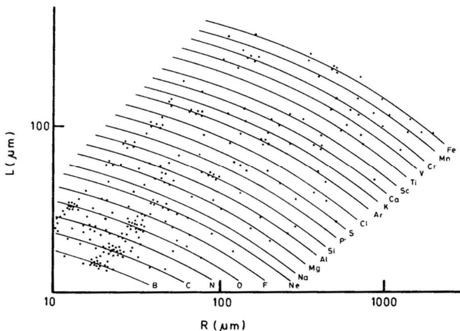
**Figure 1.** Plot of cone length ( $L$ ) versus residual range ( $R$ ).
