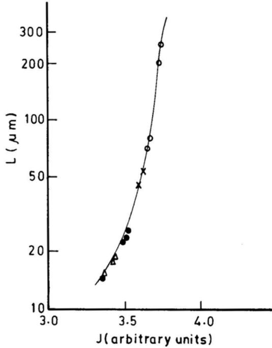
**Figure 2.**  $L$ - $J$  (Calibration curve). Triangles: carbon; filled circles: oxygen; crosses: magnesium; open circles: iron.
