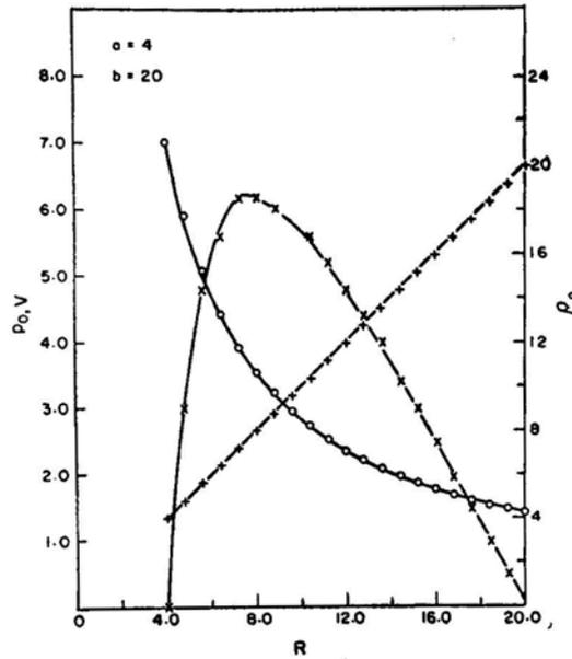
**Figure 3.** Profiles of pressure, density and velocity at  $\theta = \pi/2$  plane for the disk described in Fig. 1; (+ : density,  $\circ$  : velocity  $V_0 \times 10$ ,  $\times$  : pressure  $P_0 \times 20$ ).
