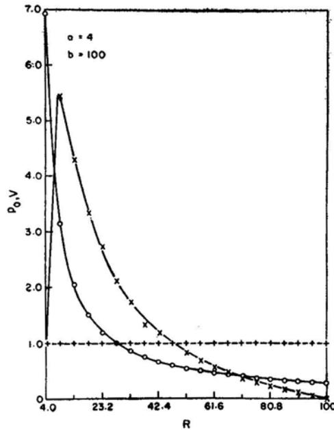
**Figure 4.** Profiles of pressure, density and velocity at  $\theta = \pi/2$  plane for the disk described in Fig. 2; (+ : density,  $\circ$  : velocity  $V_0 \times 10$ ,  $\times$  : pressure  $P_0$ ).
