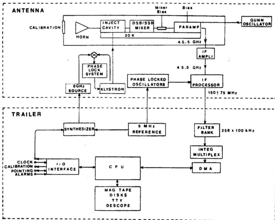
Figure 1. Block diagram of receiving system,
