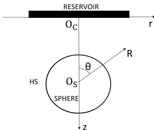
Figure 1. A cross-section of the 3D model with a uniform circular reservoir resting on a porous-elastic half space (HS) with an embedded sphere of a different porous-elastic solid. Also shown are the cylindrical  $(r, z)$  and spherical  $(R, \theta)$  coordinate systems used.
