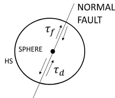
Figure 2. A normal fault intersecting the spherical inclusion. The destabilizing shear stress ( $\tau_d$ ) and the stabilizing frictional stress ( $\tau_f$ ) on the fault are also shown schematically.
