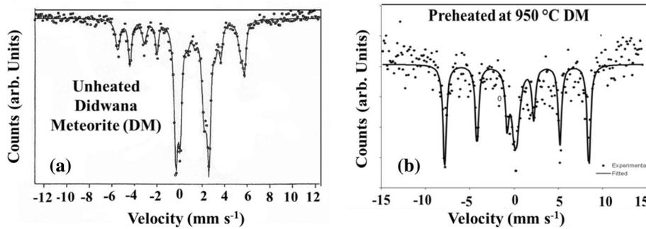
Figure 1. Mossbauer spectra of (a) unheated and (b) preheated at 950°C Didwana meteorite (DM).
