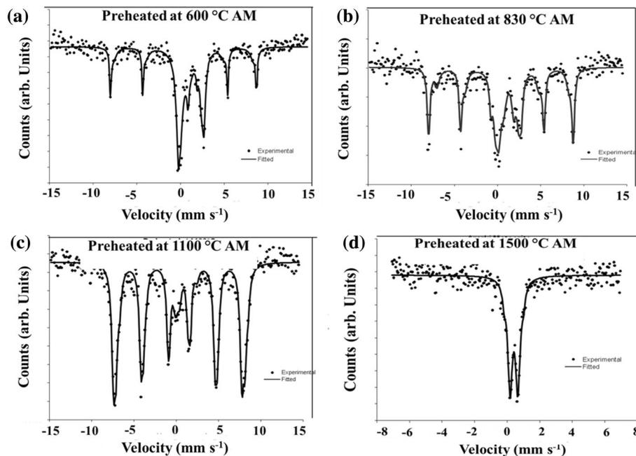
Figure 4. The Mossbauer spectra of Ararki meteorite subjected to different temperatures under ambient conditions, (a) 600°C, (b) 830°C, (c) 1100°C, and (d) 1500°C.
