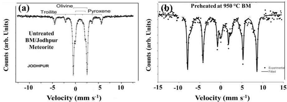
Figure 3. Mossbauer spectra of (a) unheated and (b) preheated at 950°C BM/Jodhpur meteorite (BM).
