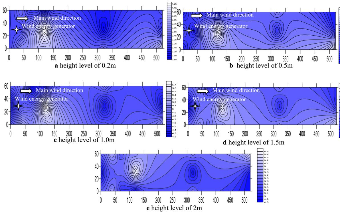
Figure 4. Horizontal distribution pattern of wind velocity at different vertical height near the surface.
