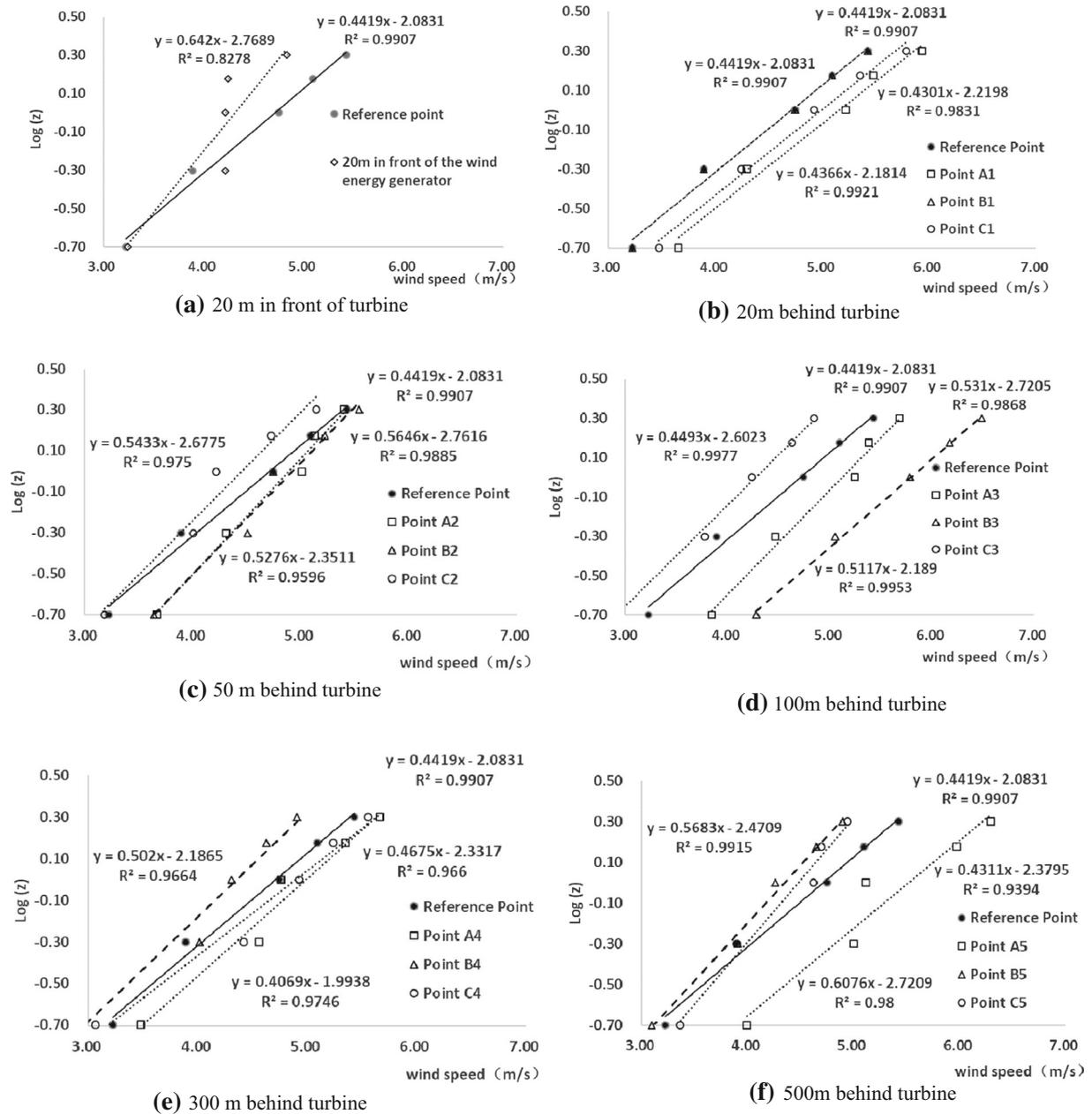
Figure 3. Fitting of the linear and logarithmic functions of wind velocity profile with different distance from wind turbine. The observed height of wind speed at each measuring point is 0.2, 0.5, 1, 1.5, and 2m.
