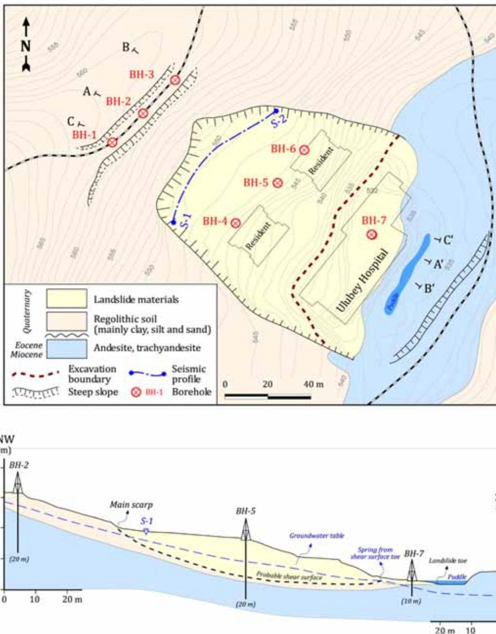
Figure 5. 1/2500 scaled engineering geological map and geological cross-section of the landslide area.
