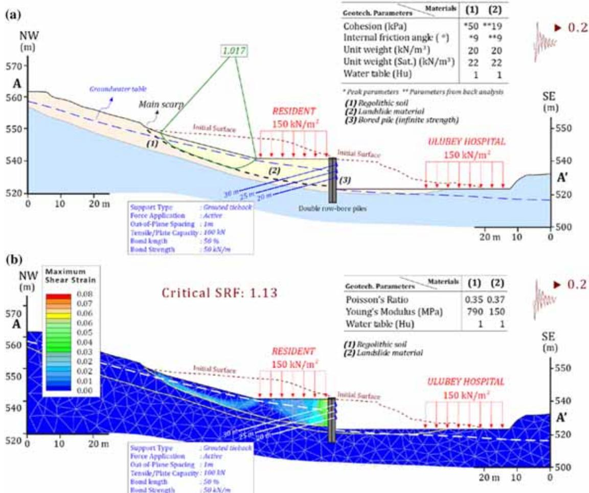
Figure 7. LE (a) and 2D-FEM-SSR (b) analyses evaluated for pseudo-static condition along the A–A' cross-section.
