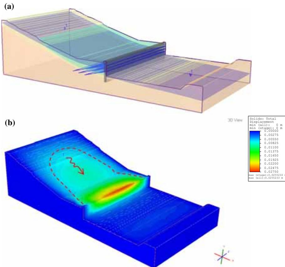
Figure 8. 3D-FEM-SSR analysis result evaluated for pseudo-static condition.
