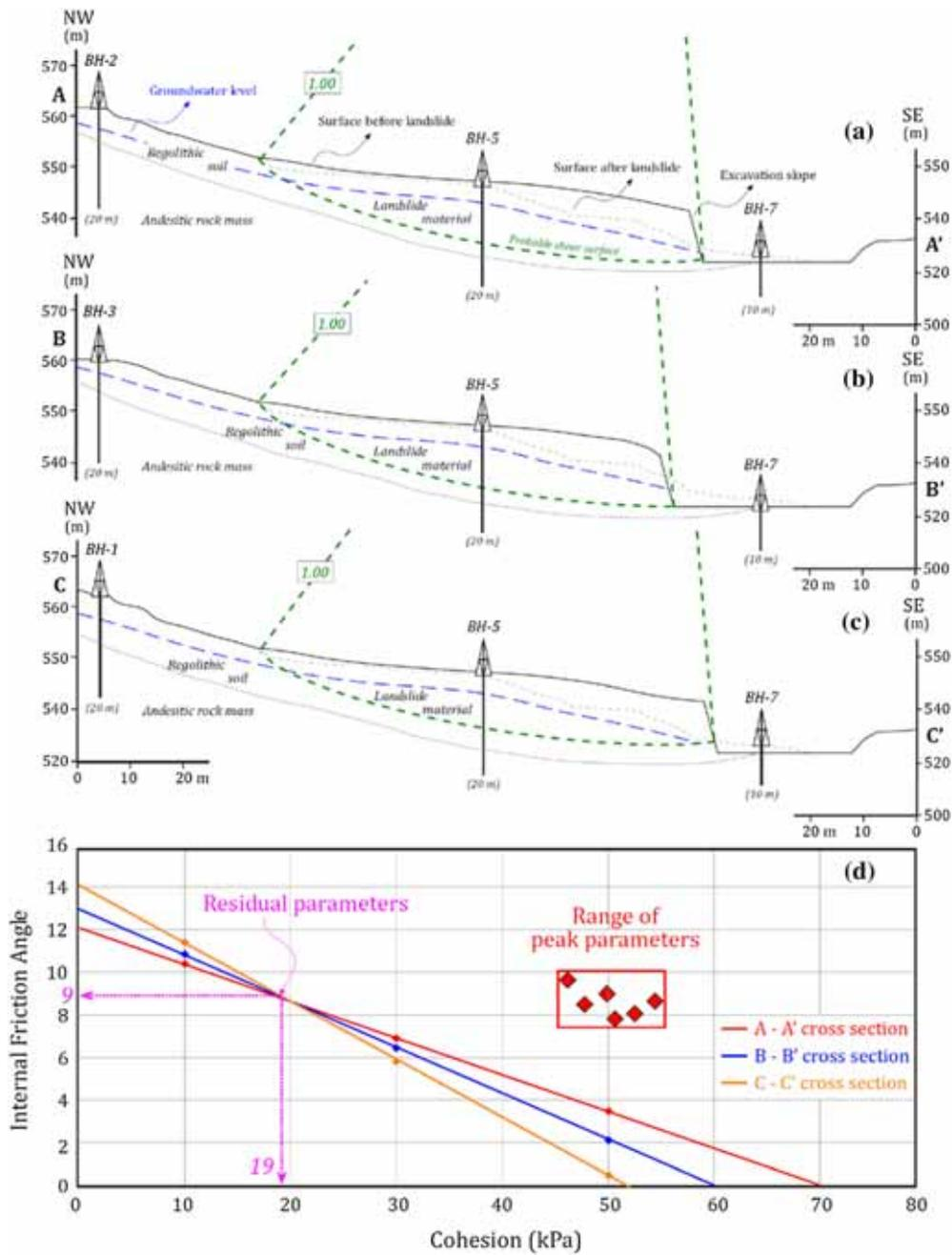
Figure 6. Back analysis carried out on three different geological cross-sections and the obtained residual parameters.
