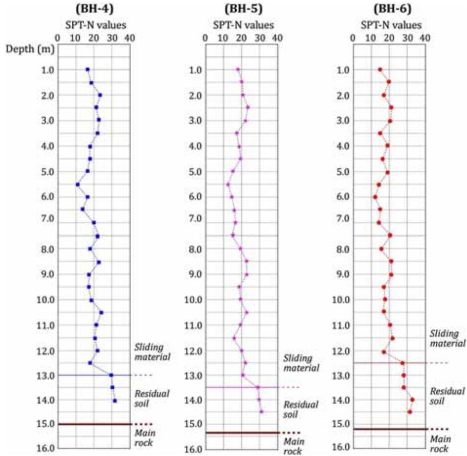
Figure 4. Results of SPT conducted in some boreholes.
