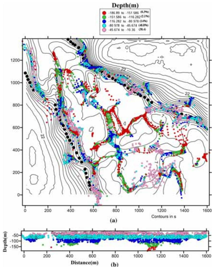
Figure 6. (a) Euler solution of conductance map of sub-vertical fault. The tightest cluster was obtained for SI 0.6. The black filled circles show the fault mapped by Kilenyi and Szabo (1985). The contour shows conductance. (b) Depth distribution of cluster Euler solution on x-z plane. The index shows the depth range along with % of solutions in the specified range.
