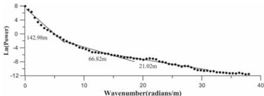
Figure 7. Radially averaged power spectrum of conductance of figure 6.
