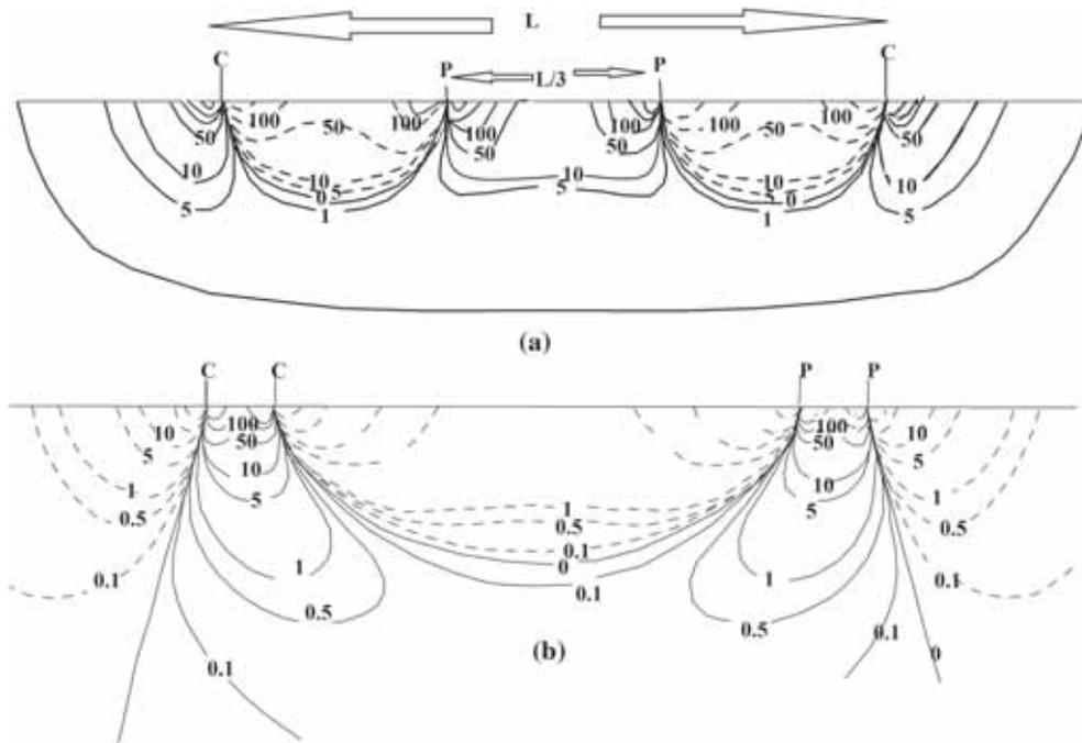
Figure 1. Signal contribution section for (a) Wenner array and (b) dipole–dipole array. Contours show the signal contribution; continuous and discontinuous lines shows for positive and negative contributions, respectively.
