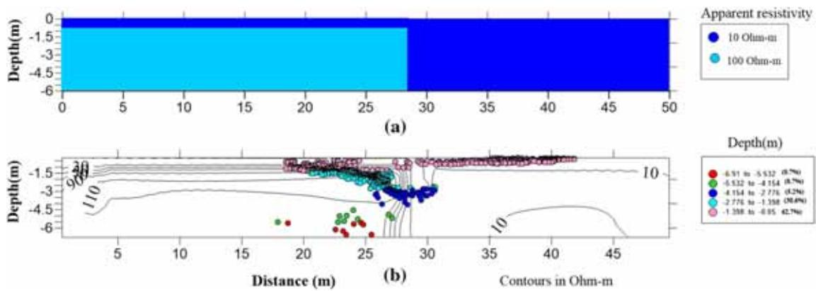
Figure 4. (a) Vertical fault model and (b) Euler depth solution of vertical fault with SI 0.6 for dipole-dipole array. The index shows the depth range along with % of solutions in the specified range.
