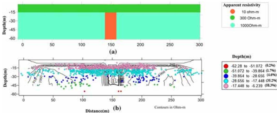
Figure 2. (a) Dyke model and (b) Euler depth solution of dyke with SI 1 for Wenner array superimposed over the inverted model resistivity section. This shows the depth range along with % of solutions in the specified range.
