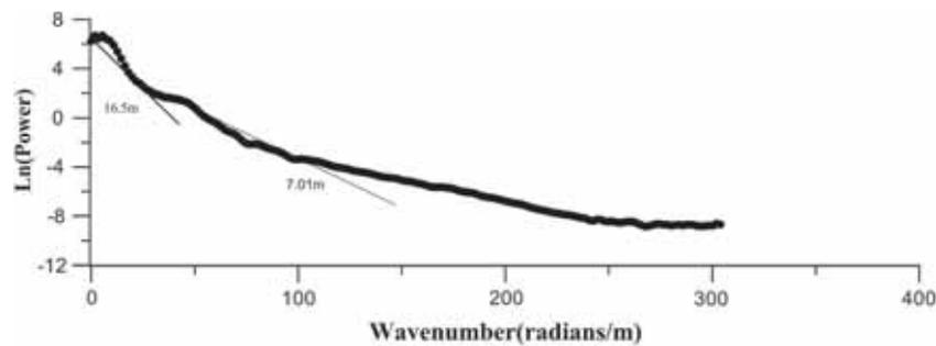
Figure 10. Radially averaged power spectrum of apparent resistivity data for Line 4 for Dhanjori data.
