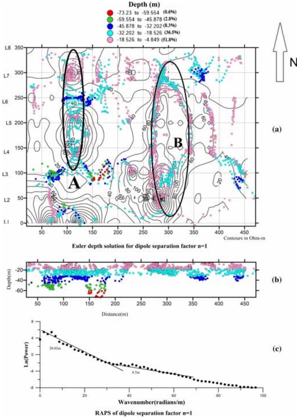
Figure 8. Euler depth solutions (top), depth distribution of clustered Euler solutions (middle) and RAPS (bottom) for dipole separation factor (a–c)  $n = 1$ , (d–f)  $n = 3$ . The index shows the depth range along with % of solutions in the specified range. L1 , . . . , L8 are the eight ERT lines along which the data have been acquired.
