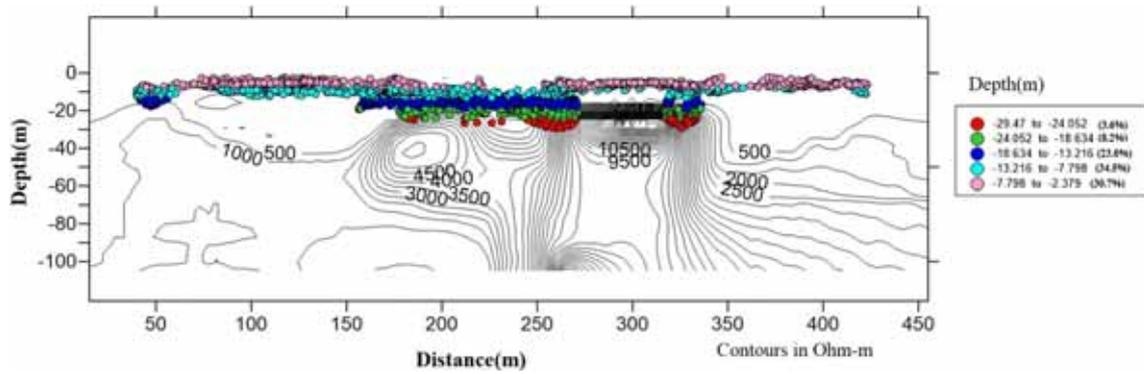
Figure 9. Euler depth solution of apparent resistivity superimposed on inverted model resistivity section for Line 4. The index shows the depth range along with % of solutions in the specified range.
