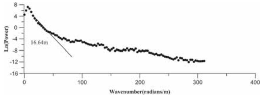
Figure 3. Radially averaged power spectrum of resistivity data for model figure 2(a).
