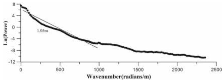
Figure 5. Radially averaged power spectrum of resistivity data for model figure 4(a).
