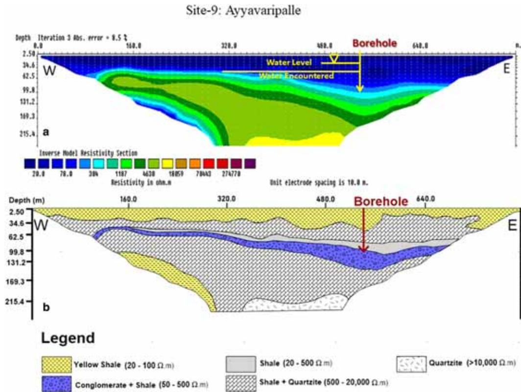
Figure 7. (a) 2D inverted resistivity model at site-9 showing low resistivity at near surface layers followed by high resistivity until the bottom depth of the section, a high yielding borehole was drilled towards eastern side of the section; (b) conceptual geological model depicting shale, quartzite and conglomerate formation. The borehole encompasses shale, shale and quartzite, thin shale layer as well as conglomerate and shale layer up to 81 m depth.
