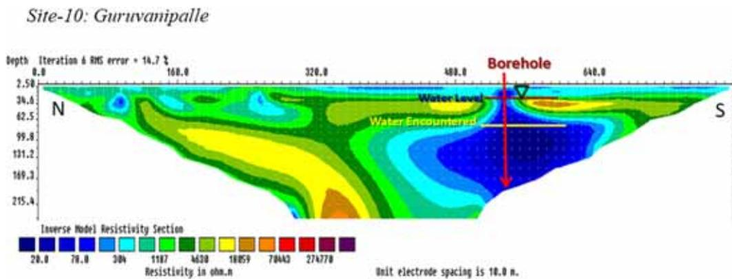
Figure 6. 2D inverted resistivity model at site-10 shows a potential groundwater zone towards southern side, which is confirmed by a drilled borehole at 535 m lateral distance. The high resistivity massive formation is delineated from 35 to 230 m towards northern side of the section with no prospect for groundwater exploration.
