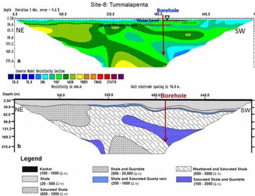
Figure 4. (a) Depicted a 2D inverted resistivity model at site-8 with a high resistivity towards the NE side and a potential zone for groundwater exploration in SW, which is confirmed by a drilled borehole at 510 m lateral distance; (b) conceptual geological model based on the 2D resistivity result depicting borehole encompasses shale, quartzite and saturated shale and quartzite formation in the entire geological strata up to 192 m depth.
