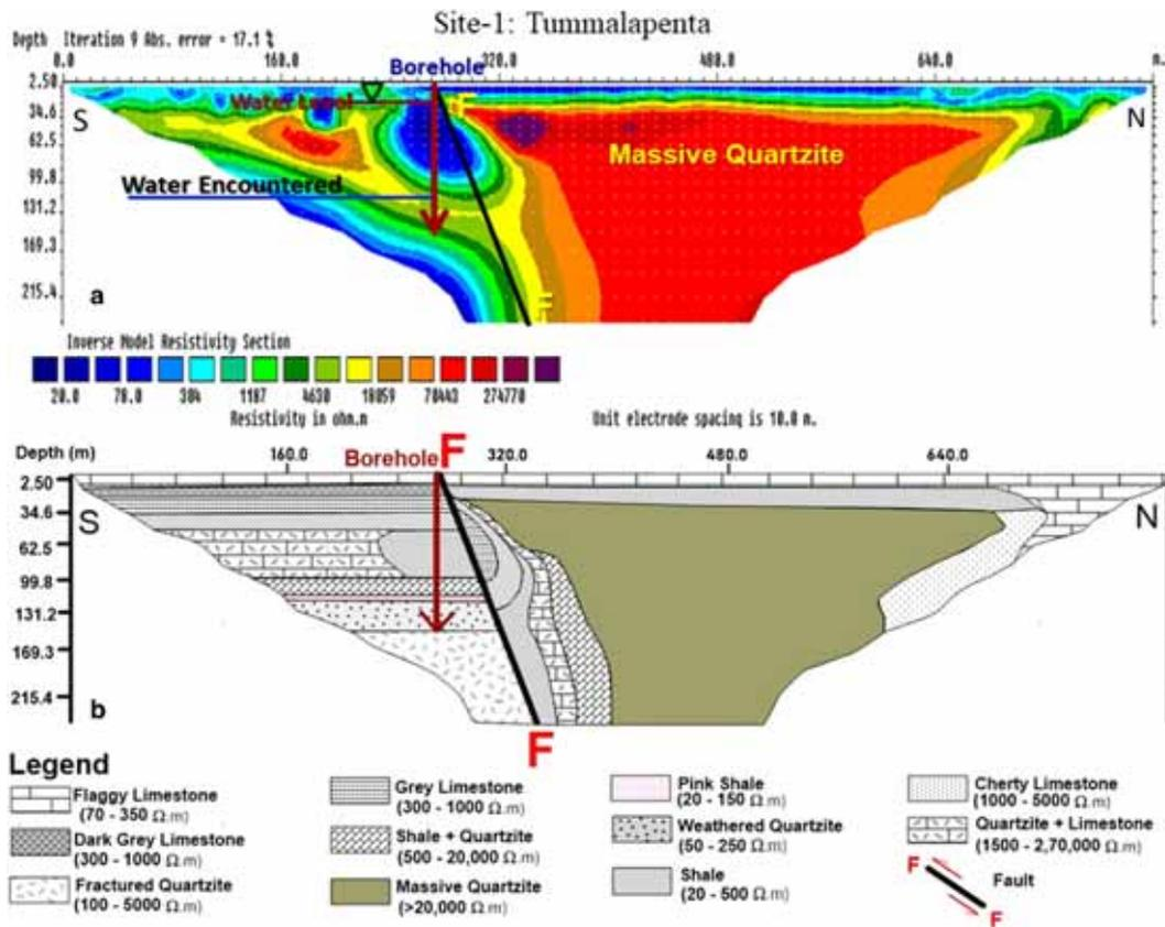
Figure 3. (a) 2D inverted resistivity model at site-1, which shows a large resistivity contrast, delineated a major fault (F-F) structure and the groundwater potential zone towards the southern side near the fault; (b) depicted the geological model, main fault structure, borehole and the thick massive quartzite rock towards the north of the fault plane.
