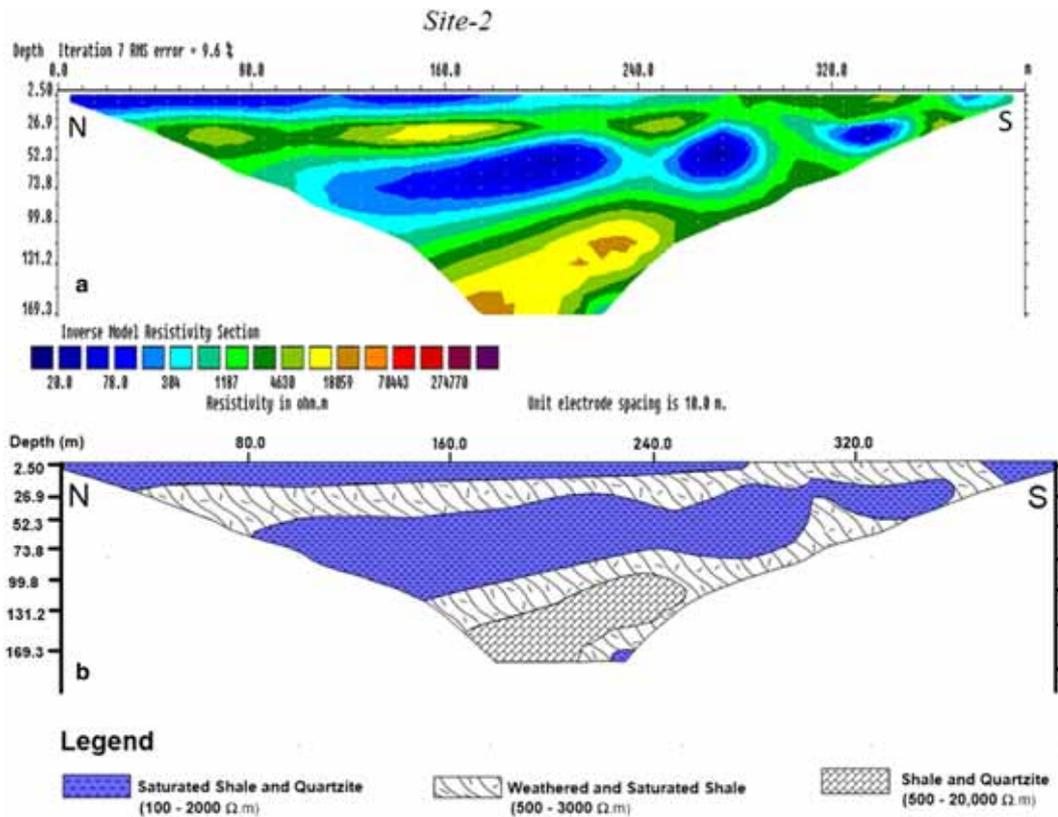
Figure 5. (a) Depicted a 2D inverted resistivity model at site-2, which revealed a heterogeneous subsurface of the geological formation with a large range of resistivity variation from the near surface layers to depths; (b) depicted the geological model based on the resistivity result, which revealed a prospect groundwater zone in saturated shale and quartzite formation.
