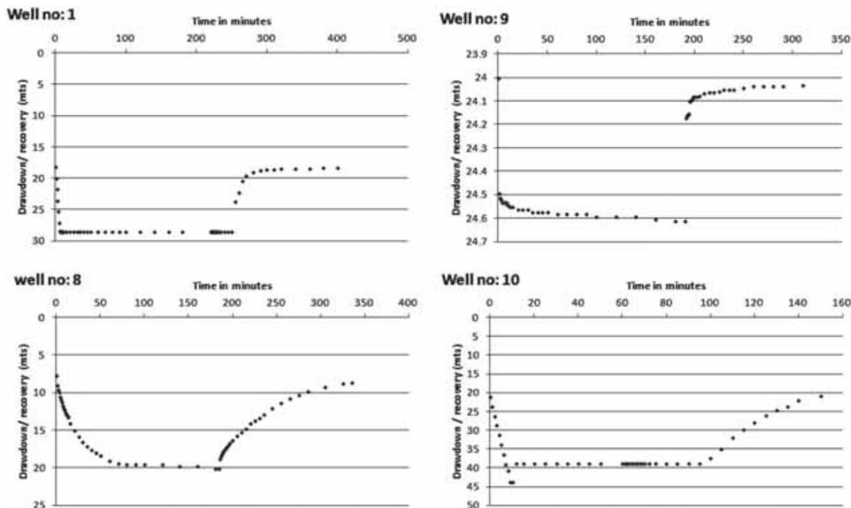
Figure 9. Drawdown and recovery curves of the four newly drilled boreholes in the area of study.
