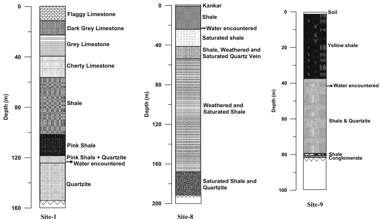
Figure 8. Detailed lithology of the drilled boreholes namely at site-1, 8 and 9 and its validation showing the water encountered at the contact zone(s) of shale and quartzite rocks as well as in the weathered shale formation.
