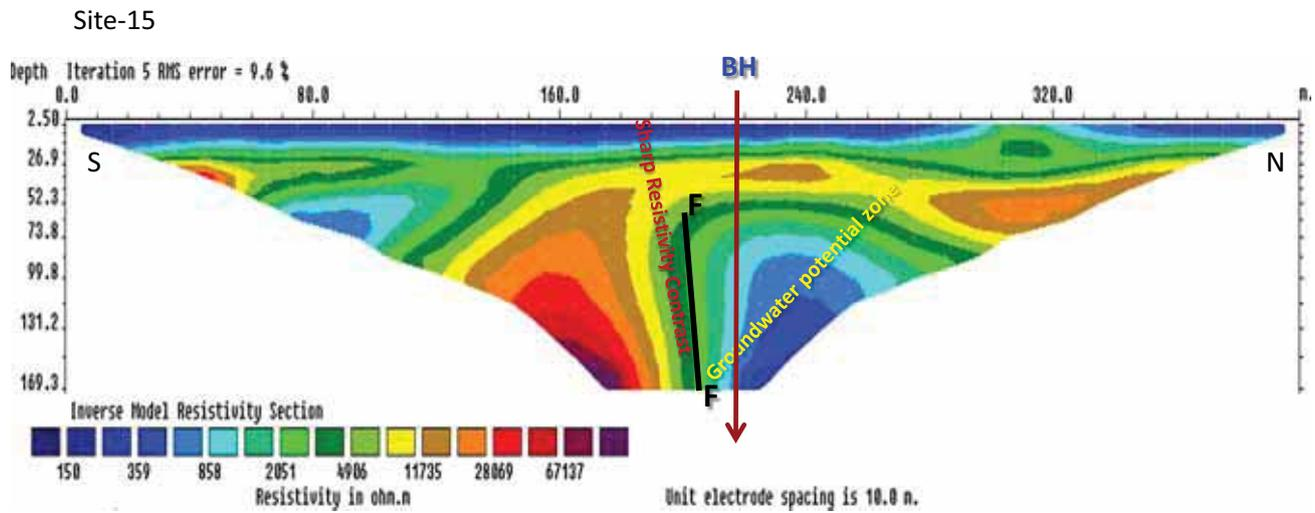
Figure 8. Shows the 2D inverted resistivity model which revealed a high and a low resistivity geological formation, which is inferred as the fault (F-F) with a prospect groundwater zone towards the right of the fault at site no. 15.
