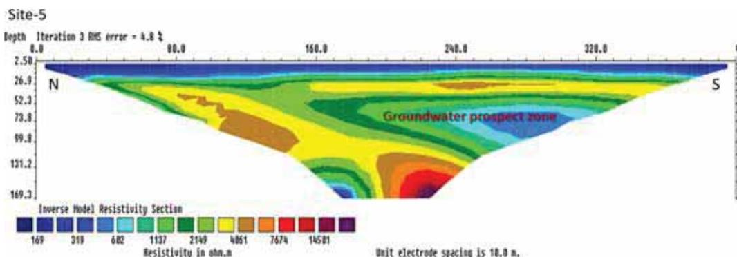
Figure 4. The figure depicts the 2D inverted resistivity model showing heterogeneous subsurface, high resistivity as well as groundwater prospect zone towards south of the section at site no. 5.
