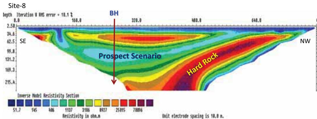
Figure 6. Depicted the 2D inverted resistivity model with clear-cut delineation of high resistivity geological structure inclined towards NW and a prospect groundwater zone sandwiched between high resistivity rock mass at site no. 8.
