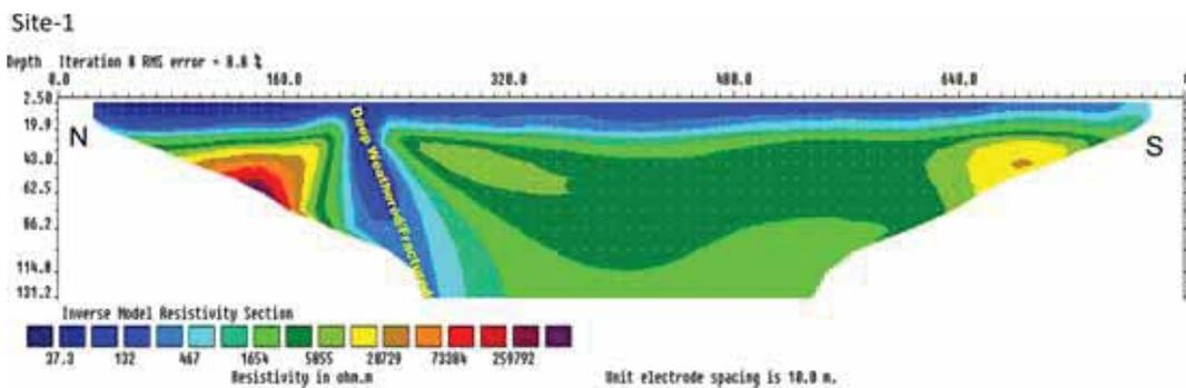
Figure 3. 2D inverted resistivity model with large resistivity contrast showing the prospect groundwater zone towards the northern side of the resistivity section at site no. 1.
