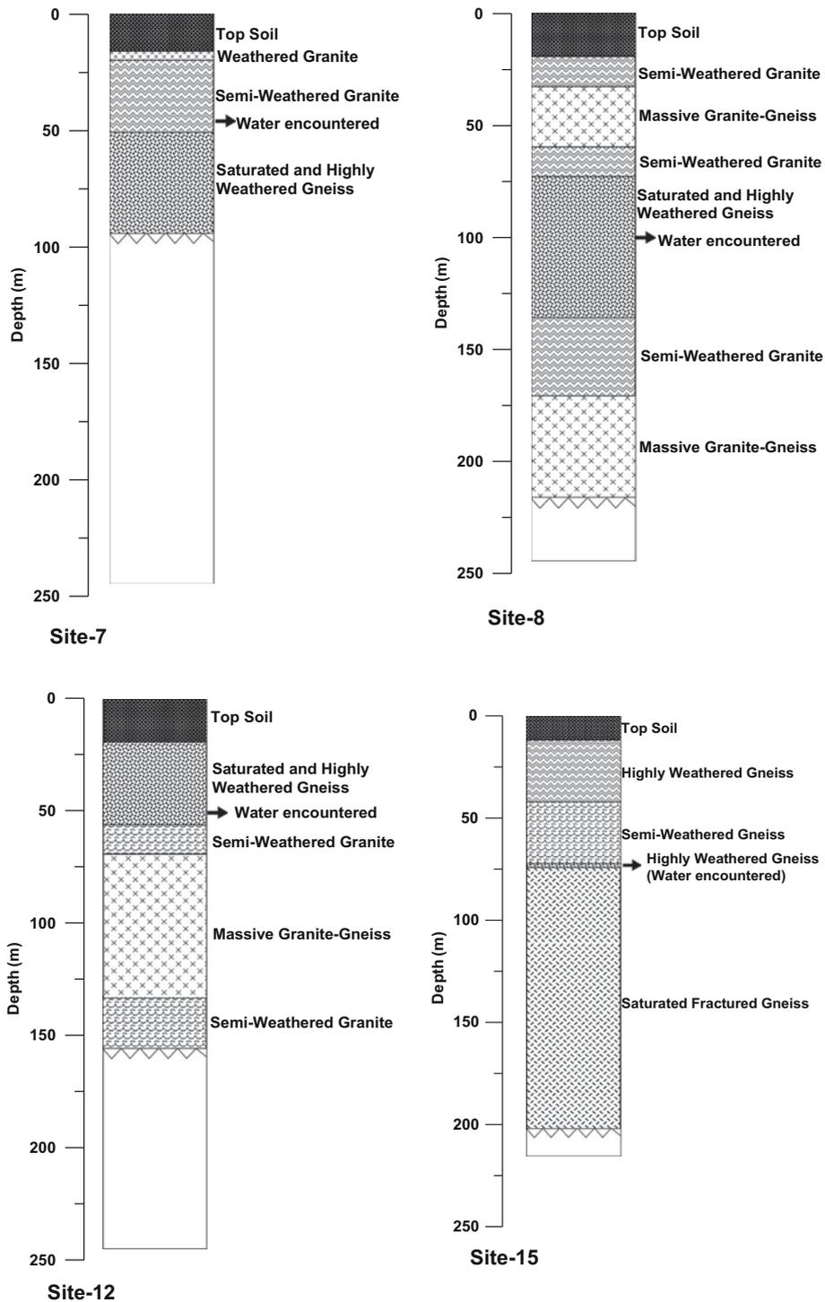
Figure 9. Detailed lithology of the drilled boreholes namely at sites 7, 8, 12 and 15 and its validation showing the water encountered at semi-weathered granite, saturated and highly weathered gneiss and highly weathered gneiss of the granite-gneiss hard rock aquifer system.
