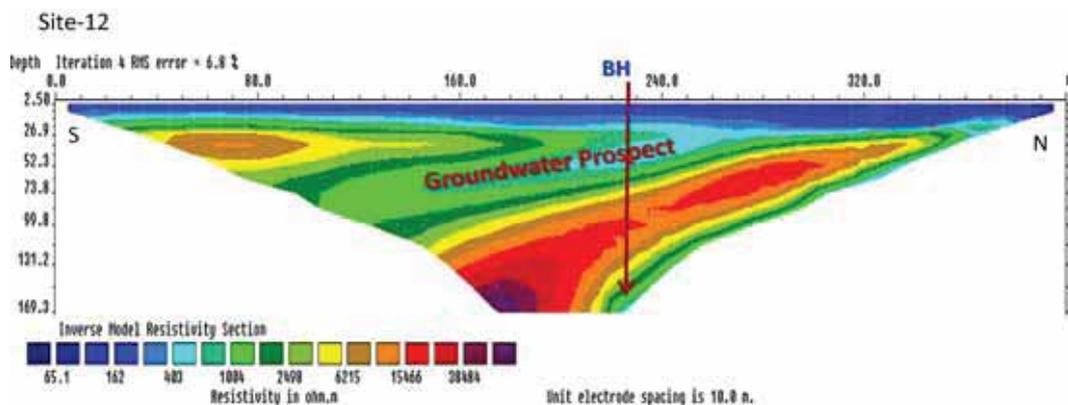
Figure 7. Depicted the 2D inverted resistivity model with a large resistivity contrast of the geological formation and delineated prospect groundwater zone between 50 and 70 m depth lying within the lateral distance 160 and 240 m at site no. 12.
