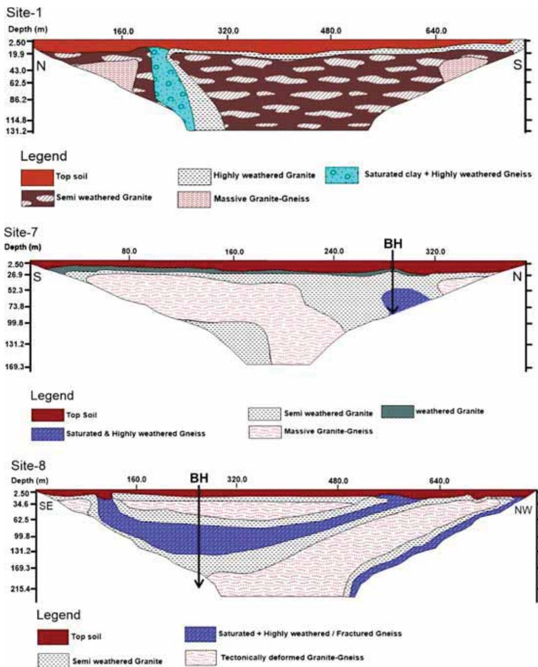
Figure 10. Depicted the conceptual geological models at sites-1, 7, 8, 12 and 15 arrived based on the 2D resistivity results, borehole lithology data and the geological setting of the Chhotanagpur granite-gneiss of Chhotanagpur Gneissic Complex (CGC) region.
