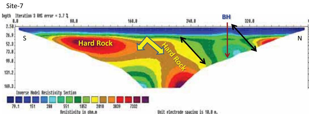
Figure 5. Shows the 2D inverted resistivity model where the northern side of the resistivity section shows more prospects for groundwater exploration as compared to the southern side at site no. 7.
