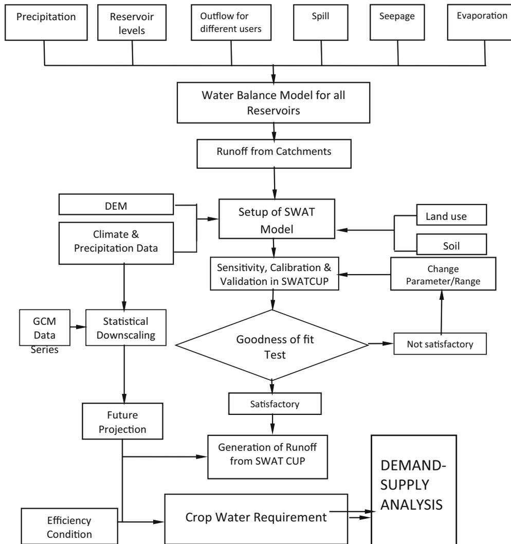
Figure 2. Work flow for proposed methodology under RDM framework.
