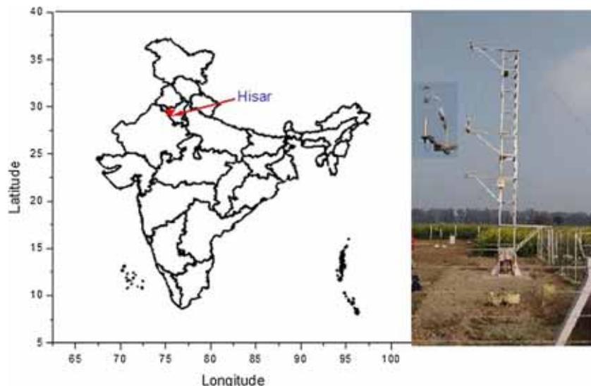
Figure 1. Location of Hisar site and Eddy covariance system installed at 6 m height on tower.
