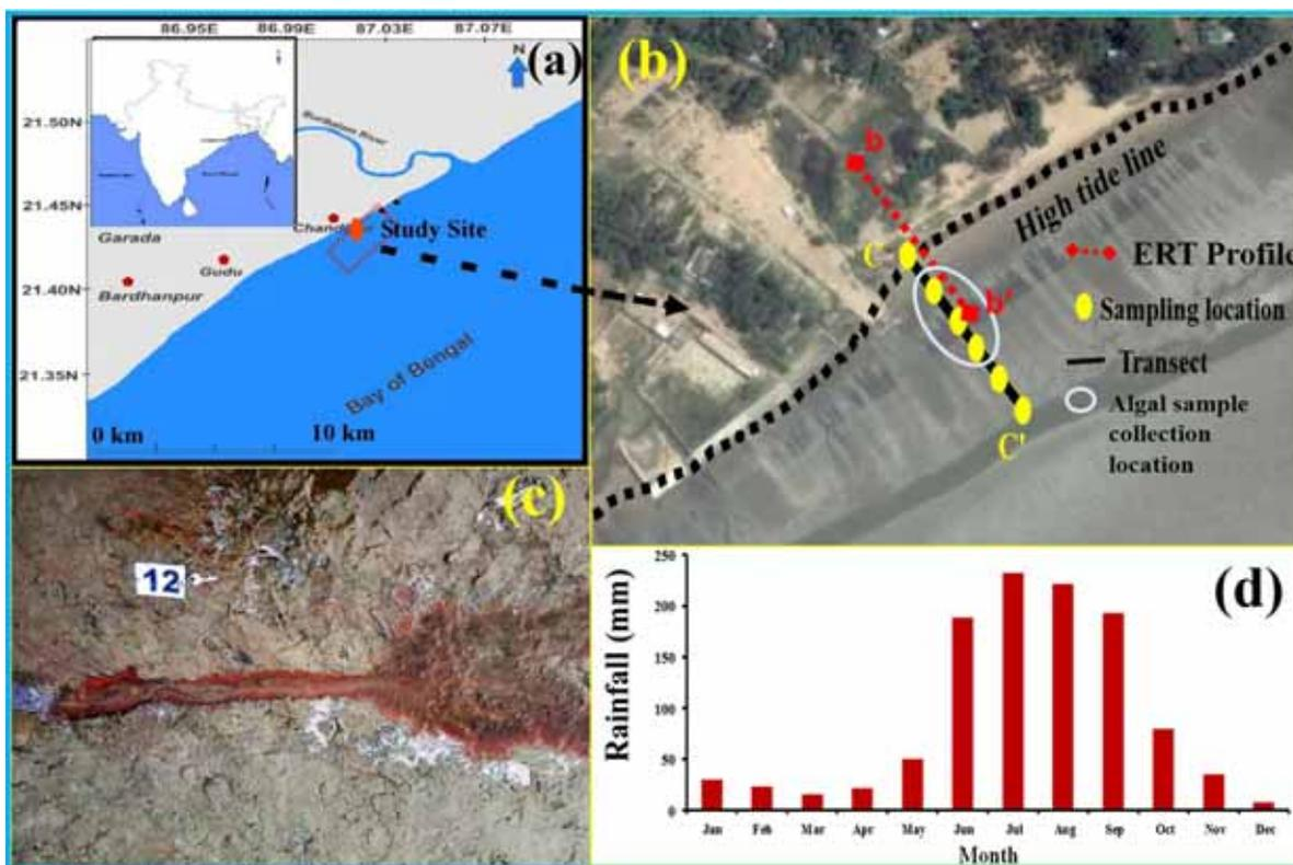
Figure 1. (a) Geographic location of the study site with location details (modified after Debnath *et al.* 2018). (b) Aerial view of the study sites with sampling locations of ERT profile (b–b'), SGD samples (both porewater and seepage water) (C–C') and algal samples. (c) Representing the focused seepage point of respective study area with iron stain. (d) Monthly average rainfall distribution of last 36 yrs (1979–2015) of Chandipur, Orissa (modified after Debnath *et al.* 2018).
