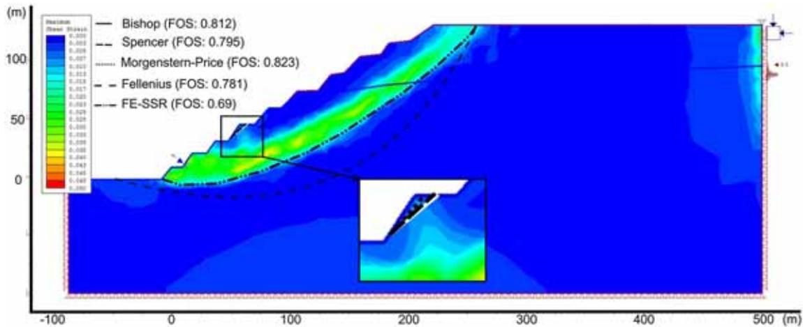
Figure 3. The failure surfaces detected by the LEMs and FE-SSR for slope model-1, while GSI: 35, slope angle: 30°, WTL: 50%, seismic coefficient: 0.3 g.
