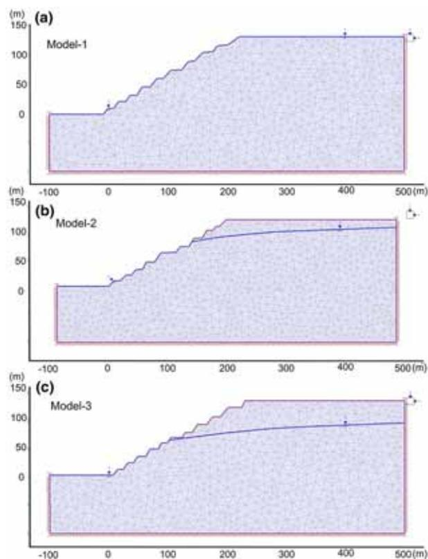
Figure 1. The Phase<sup>2</sup> models of three slopes with different heights adapted from Kadakci (2011) showing (a) fully saturated (100%) Model-1, (b) partially saturated (70%) Model-2, and (c) partially saturated (50%) Model-3.
