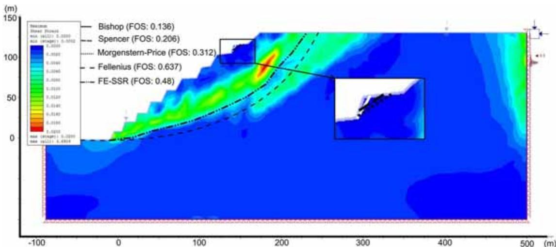
Figure 6. The failure surfaces detected by the LEMs and FE-SSR for slope model-1, while GSI: 35, slope angle:  $36^\circ$ , WTL: 100%, seismic coefficient: 0.3 g.
