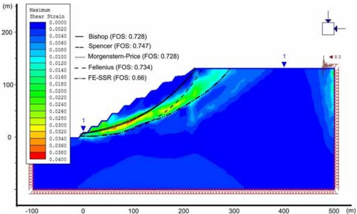
Figure 4. The failure surfaces detected by the LEMs and FE-SSR for slope model-1, while GSI: 35, slope angle: 30°, WTL: 100%, seismic coefficient: 0.3 g.
