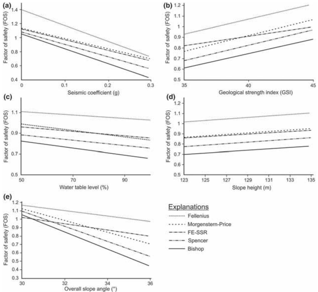
Figure 2. Variations of FOS values for different (a) seismic coefficients, (b) GSI ratings, (c) water table levels, (d) slope heights, and (e) overall slope angles.
