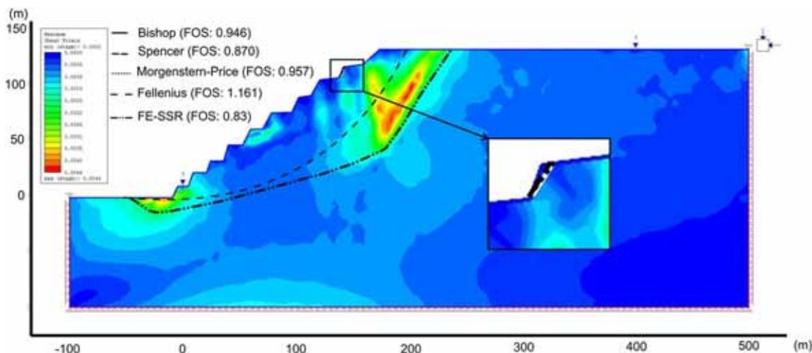
Figure 5. The failure surfaces detected by the LEMs and FE-SSR for slope model-1, while GSI: 35, slope angle:  $36^\circ$ , WTL: 100%, seismic coefficient: 0.
