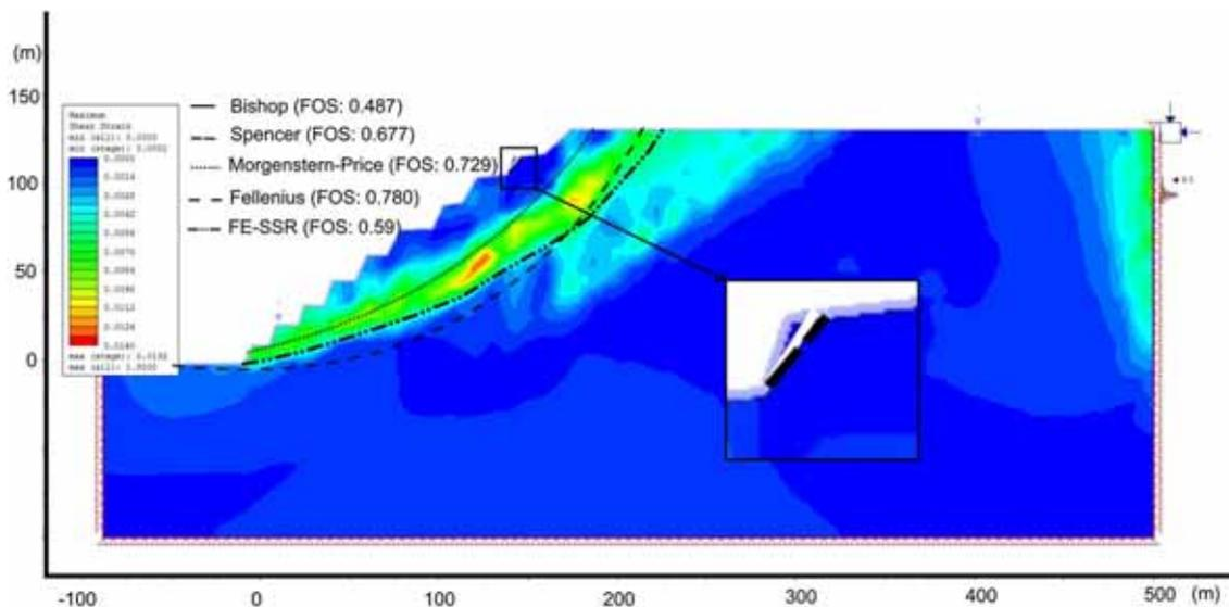
Figure 7. The failure surfaces detected by the LEMs and FE-SSR for slope model-1, while GSI: 45, slope angle: 36°, WTL: 100%, seismic coefficient: 0.3 g.
