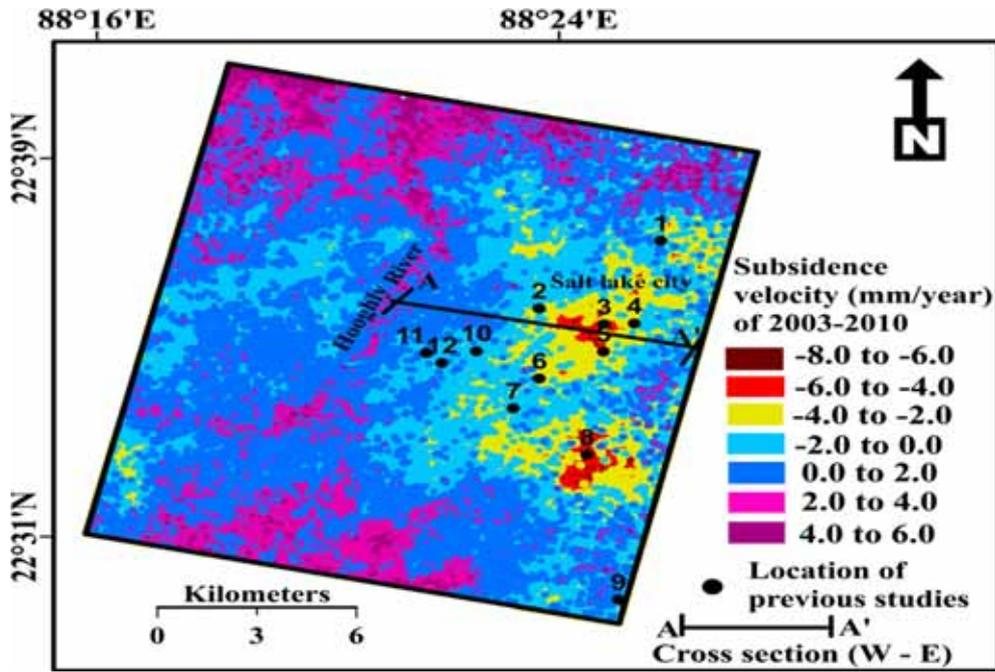
Figure 4. Velocity of subsidence rates measured over the period from the year 2003 to 2010 (negative values stand for relative subsidence).
