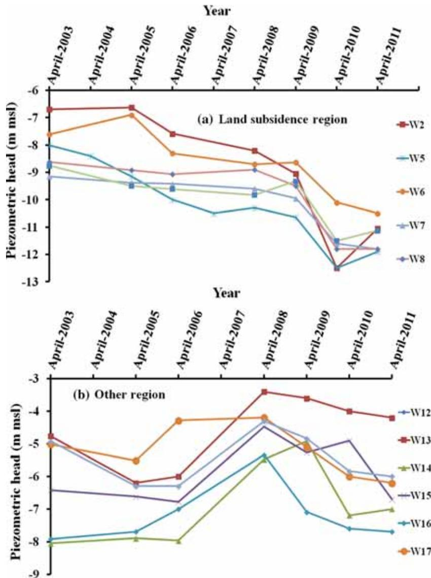
Figure 7. Year wise changes in the piezometric head in piezometers during the month of April in (a) land subsidence region and (b) other regions.
