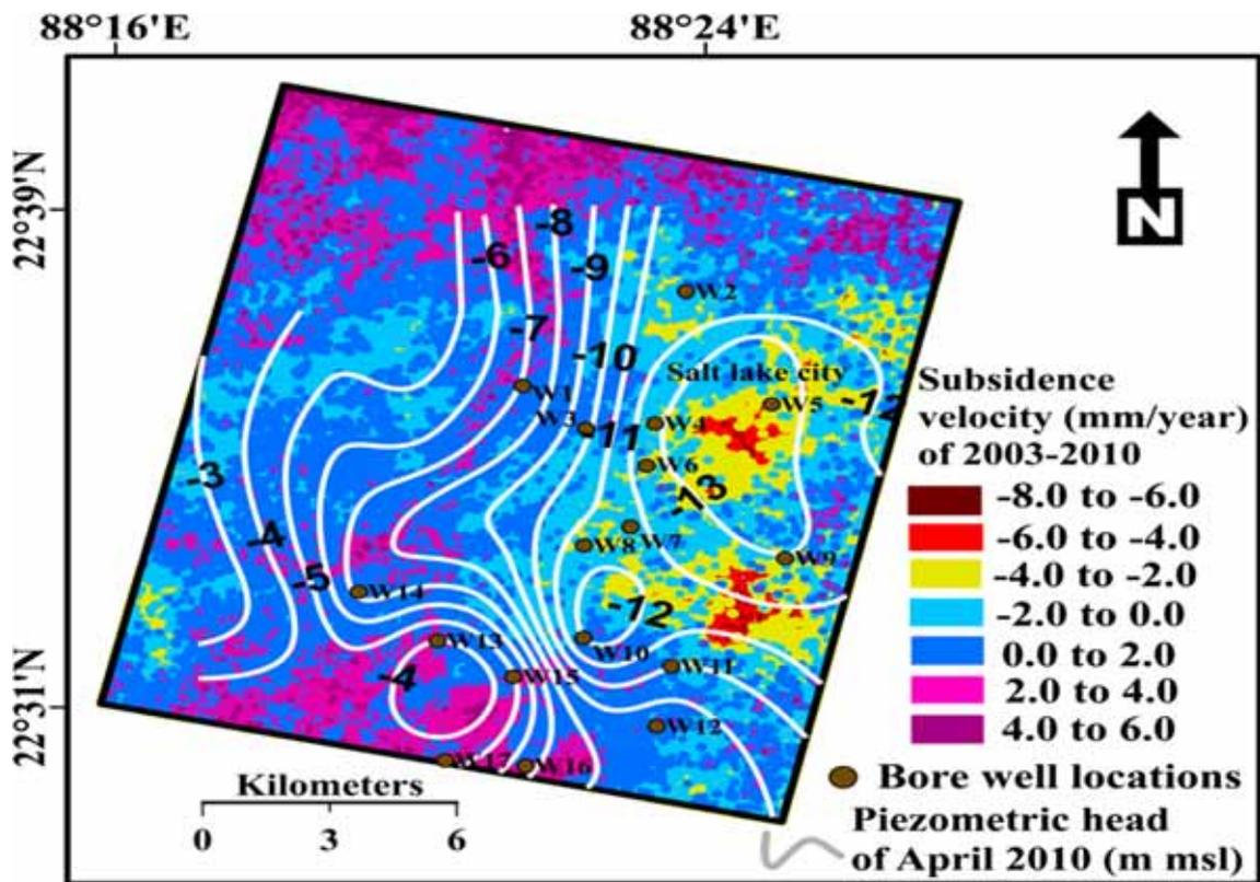
Figure 9. Variation in piezometric head overlaid on land subsidence velocity map.
