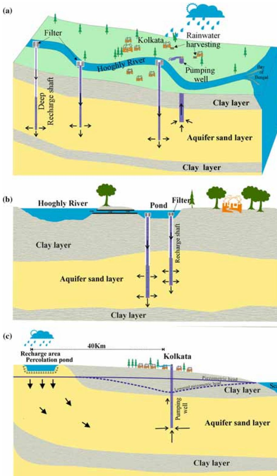
Figure 11. Conceptual diagrams showing remedial measures: (a) recharge shafts in the Hooghly river, (b) river water recharge through pond concept of UTFI (Pavelic *et al.* 2012), and (c) percolation pond in the recharge area.
