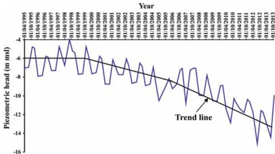
Figure 6. Changes of the groundwater level in the Salt Lake City (CGWB 2014).
