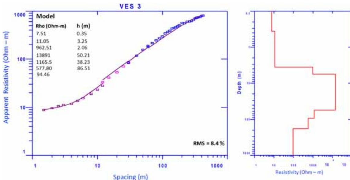
Figure 6. Shows the vertical electrical sounding (VES) model result (VES-3) where the square box is the field data and smooth line is the computed curve along with resistivity vs. depth model.
