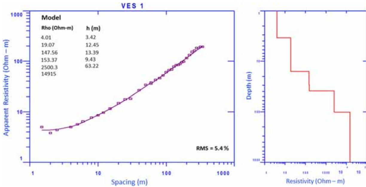
Figure 4. Shows the vertical electrical sounding (VES) model result (VES-1) where the square box is the field data and smooth line is the computed curve along with resistivity vs. depth model.
