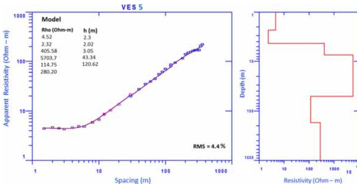
Figure 8. Shows the vertical electrical sounding (VES) model result (VES-5) where the square box is the field data and smooth line is the computed curve along with resistivity vs. depth model.
