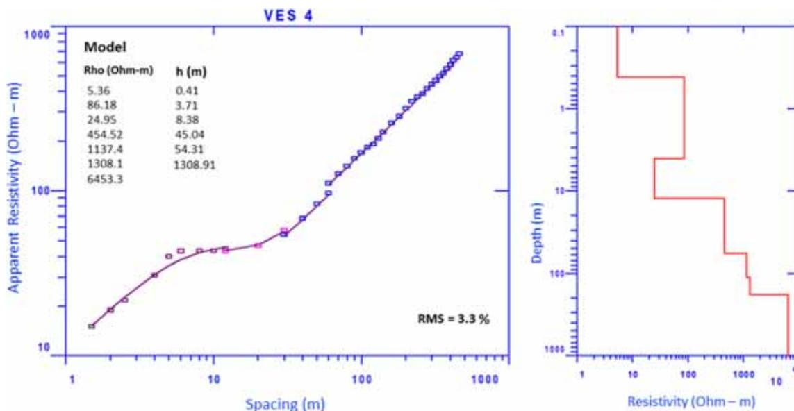
Figure 7. Shows the vertical electrical sounding (VES) model result (VES-4) where the square box is the field data and smooth line is the computed curve along with resistivity vs. depth model.
