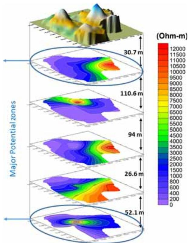
Figure 11. Shows the stacked 3D section from VES results depicting the potential layers of groundwater zones at different depth levels.
