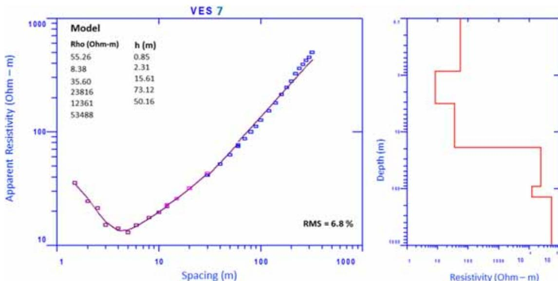
Figure 10. Shows the vertical electrical sounding (VES) model result (VES-7) where the square box is the field data and smooth line is the computed curve along with resistivity vs. depth model.
