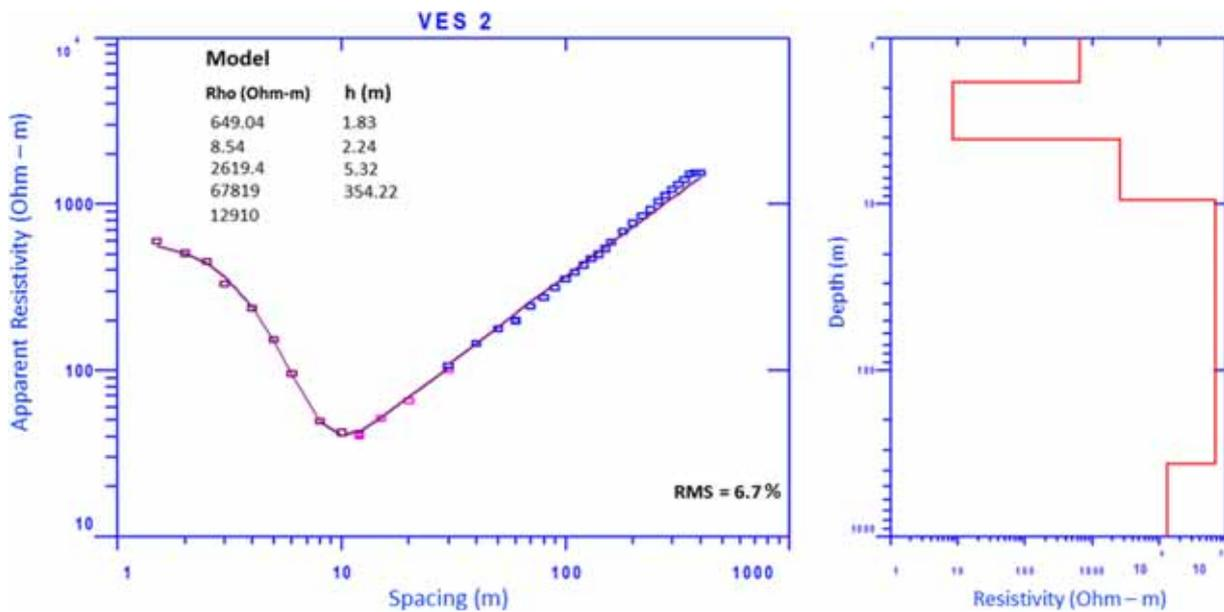
Figure 5. Shows the vertical electrical sounding (VES) model result (VES-2) where the square box is the field data and smooth line is the computed curve along with resistivity vs. depth model.
