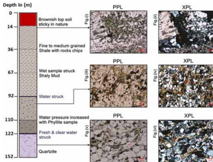
Figure 12. Shows the correlation of borehole litholog with thin sections of rock samples at different depth levels (where PPL – plane polarised light, XPL – cross polarised light).
