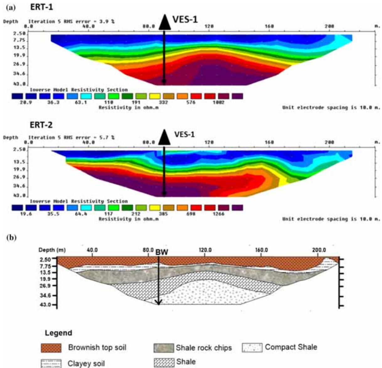
Figure 3. (a) Electrical resistivity tomography (ERT) model result near the foothill of the study area. ERT-1 is the inverted resistivity section of Wenner–Schlumberger array while ERT-2 represents dipole–dipole inverted resistivity section at the same location as shown in figure 3. (b) Conceptual geological model based on the subsurface resistivity characterization and lithology of the drilled borehole at Gundreddypalle site.
