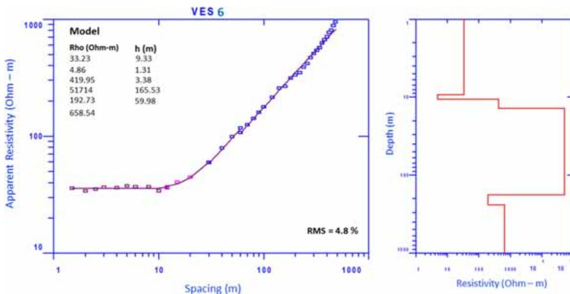
Figure 9. Shows the vertical electrical sounding (VES) model result (VES-6) where the square box is the field data and smooth line is the computed curve along with resistivity vs. depth model.
