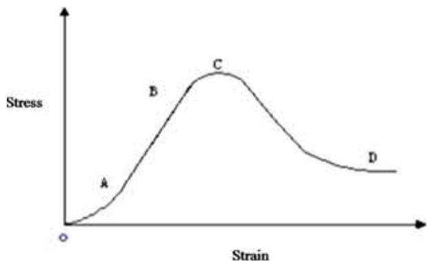
Figure 6. Stress-strain curve of coal and rock deformation and fracture.
