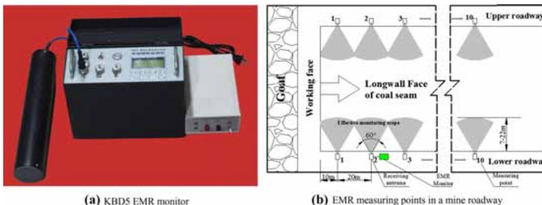
Figure 9. EMR monitoring device and measuring points layout.
