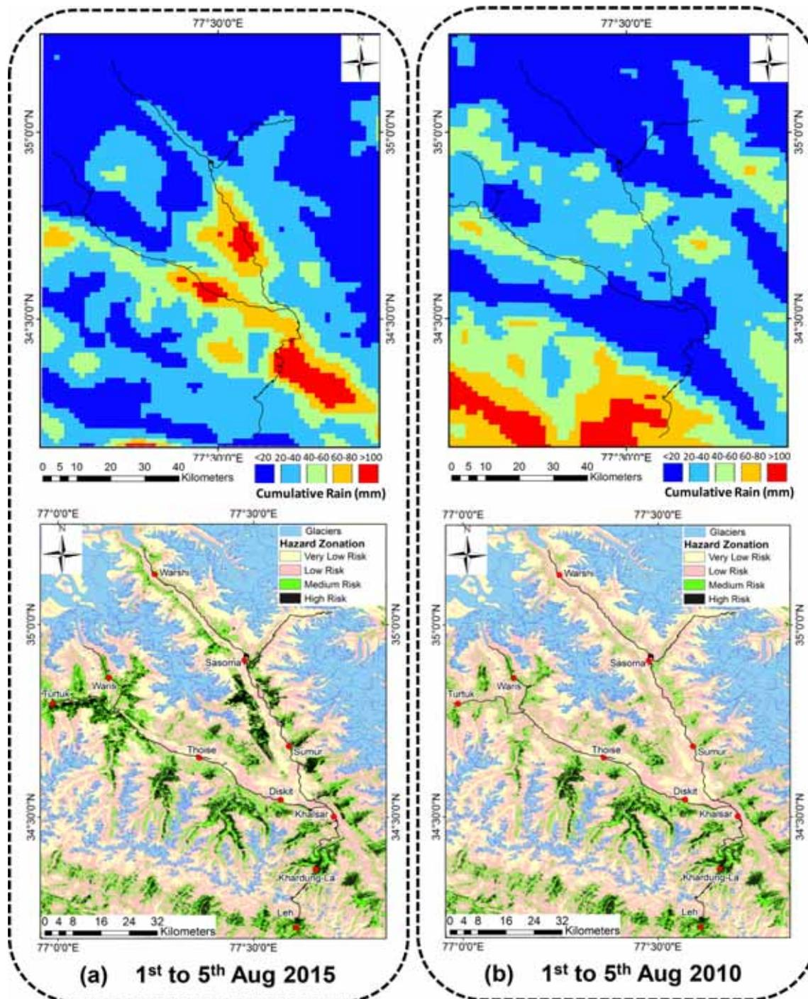
Figure 8. Two cases studies of debris flow events: (a) WRF simulation for period 1<sup>st</sup> to 5<sup>th</sup> August 2015 and corresponding susceptibility debris flow zonation; (b) WRF simulation for period 1–5<sup>th</sup> August 2010 and corresponding susceptibility debris flow zonation.
