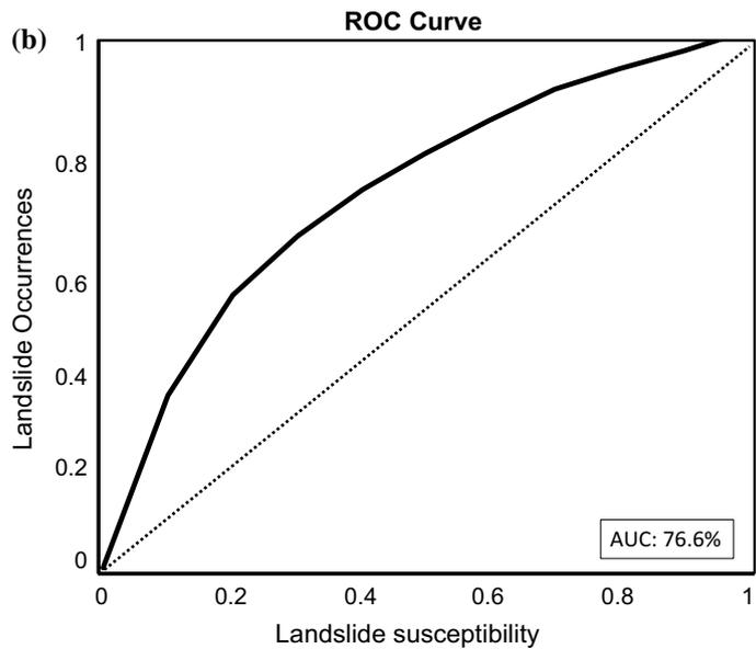
Figure 10. (a) Validation of retrieved susceptibility zones of 2015 debris flow events in Nubra valley using field survey and satellite data and (b) Assessment of susceptibility map performance for 2015 events based on ROC (normalized over both the axes).
