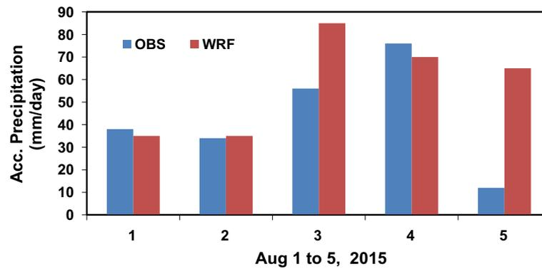
Figure 7. Comparison of WRF 5-day precipitation forecast and gauge-based rainfall observations.
