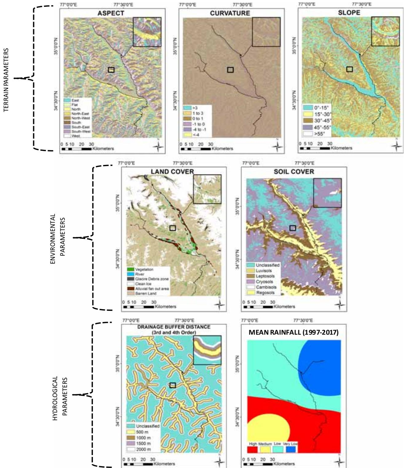
Figure 2. Thematic layers of terrain, environmental and hydrological parameters considered for mapping debris flow zones. Square black box in the figures represents the zoomed portion.
