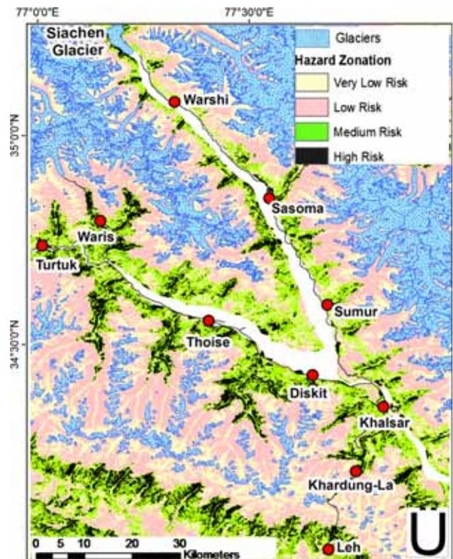
Figure 6. Map showing debris flow susceptible zones derived using weighted overlay technique.
