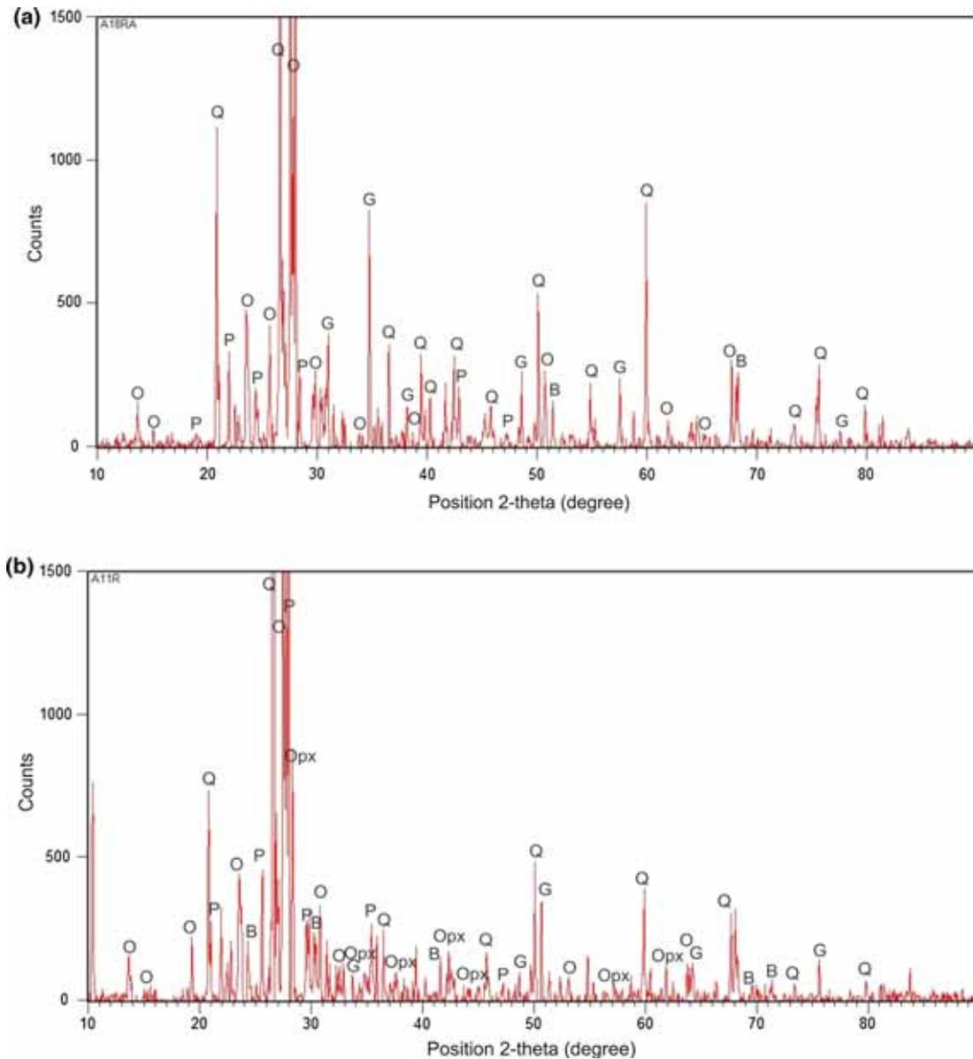
Figure 3. XRD spectra of a representative (a) QFG (A18R) and (b) charnockite (A11R) sample. Major minerals are identified from the respective peaks. Abbreviations. Q: Quartz, O: Orthoclase feldspar, P: Plagioclase feldspar, B: Biotite, G: Garnet and Opx: Orthopyroxene.
