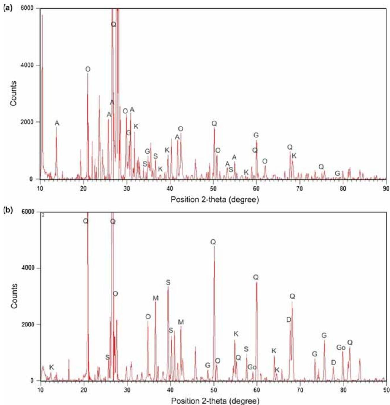
Figure 4. XRD spectra of (a) slightly weathered khondalite (Sample 16A), (b) weathered khondalite (Sample 2) and (c) extremely weathered khondalite (Sample 3B). Both major and clay minerals are identified from their respective peaks. Abbreviations. Q: Quartz, O: Orthoclase feldspar, P: Plagioclase feldspar, B: Biotite, G: Garnet, K: Kaolinite, S: Sillimanite, M: Montmorillonite, D: Diaspore, Go: Goethite, C: Cordierite and Gi: Gibbsite.
