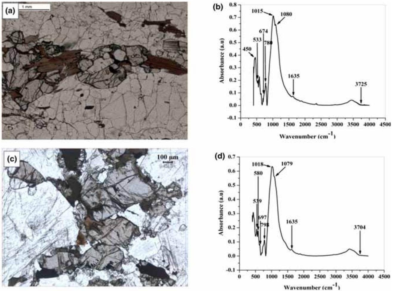
Figure 2. Photomicrographs of rock types with corresponding FTIR spectra from the study area. (a and b) Quartzofeldspathic gneiss; (c and d) Charnockite; (e and f) slightly weathered khondalite; (g and h) weathered khondalite; and (i and j) extremely weathered khondalite (for further information see the text).
