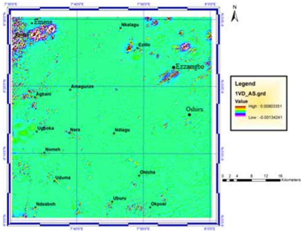
Figure 5. First vertical derivative (1VD) map of the area.
