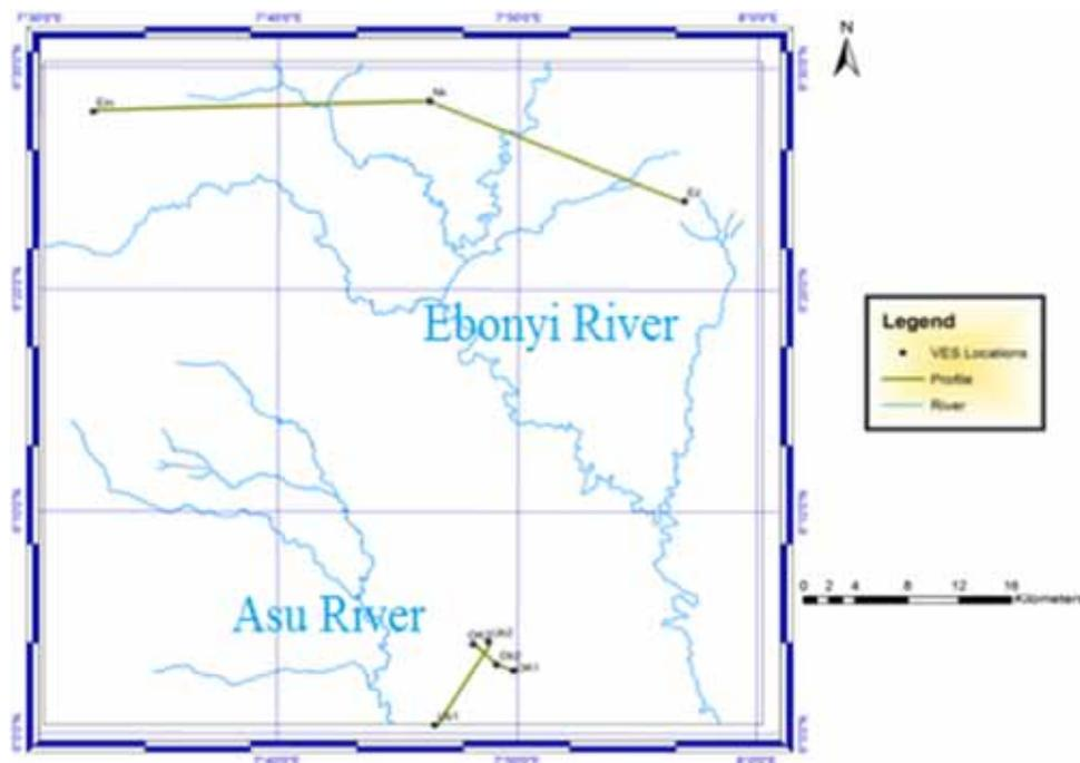
Figure 10. Drainage map of the study area with VES locations and the profile lines.
