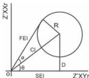
Figure 6. The image is showing the Mohr circle and its properties. The  $\tan \phi$  derived from the ratio of the radius ( $R$ ) and first effective impedance ( $FEI$ ). The ratio of Mohr circle y-coordinate ( $D$ ) and central impedance ( $CI$ ) produced  $\sin \theta$ .
