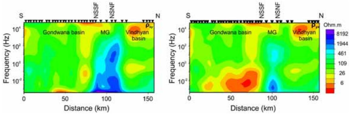
Figure 15. Pseudosections of apparent resistivity ( $\rho_{xy}$  and  $\rho_{yx}$ ) along the profile in Rewa–Shahdol region.
