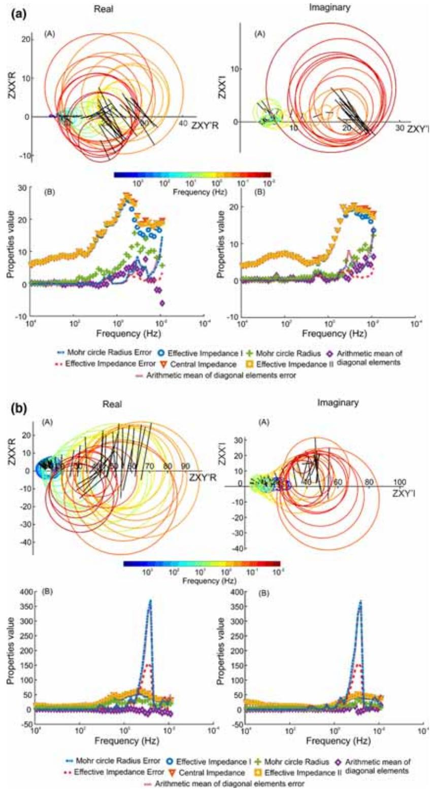
Figure 12. Real and imaginary parts of Mohr circle on common axis (figure A) and Mohr circle properties plot with respect to the frequency (figure B) for R1, R2, R3, R4 and R5 MT stations in figure 12(a–e), respectively. In figure 12d (B), the arithmetic mean of diagonal elements and Mohr circle radius values fluctuated at the 1-D condition (rectangular box).
