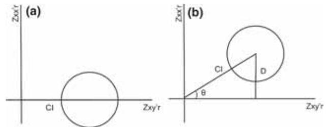
Figure 8. Representation of dimensionality using Mohr circle center point (y-coordinate or  $D$ ) and central impedance. The angle zero indicates the 1-D or 2-D structure (a) and non-zero angle obtained when the structure is 3-D (b).
