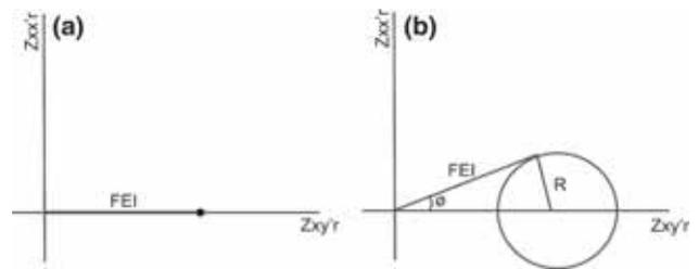
Figure 7. Representation of dimensionality using Mohr circle radius and first effective impedance. Angle zero indicates the 1-D structure (a) and non-zero angle obtained when the structure is 2-D or 3-D (b).
