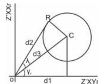
Figure 2. Real parts of first effective impedance ( $d2$ ), second effective impedance ( $d1$ ), central impedance ( $d3$ ), anisotropy angle ( $\lambda$ ) and skew angle ( $\gamma$ ) are plotted (modified after Lilley 1993a).
