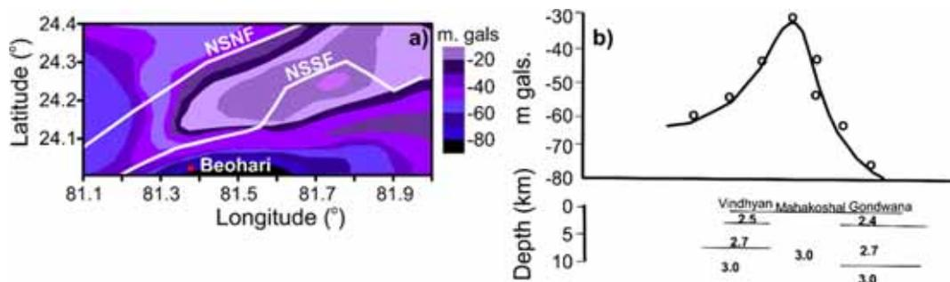
Figure 17. (a) Bouguer gravity contour map of NSL zone obtained from Qureshy and Warsi (1975) and (b) Gravity model across the profile (see the profile direction in figure 9) in the NSL zone (CRUMANSONATA 1995).
