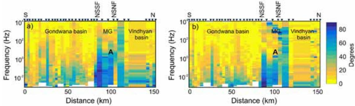
Figure 13. Pseudosection of  $\tan \phi$  (real and imaginary components) derived from the MT data from Rewa–Shahdol region. Color scale indicates the range of angle. The real component is plotted in the left (a) and the imaginary component is plotted to the right (b). The image shows high values of  $\tan \phi$  ('A' in this figure) below the NSL region comprising of NSSF and NSNF. MG: Mahakoshal Group of rocks.
