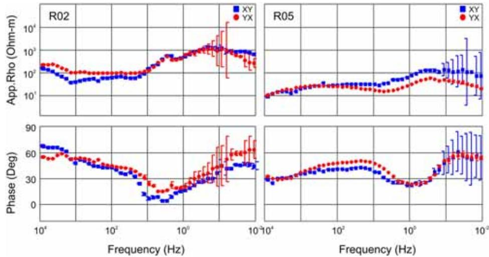
Figure 10. Apparent resistivity and phase responses of R2 and R5 stations, which are measured in geographic coordinates (X, North–South; Y, East–West).
