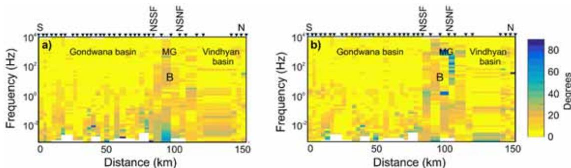
Figure 14. Pseudosection of  $\sin \theta$  (real and imaginary components) derived from the MT data from Rewa–Shahdol region. Color scale indicates the range of angle. The real component is plotted in the left (a) and the imaginary component is plotted in the right (b). High values of  $\sin \theta$  ('B' in this figure) are observed in the NSL region comprising of NSSF and NSNF. MG: Mahakoshal group of rocks.
