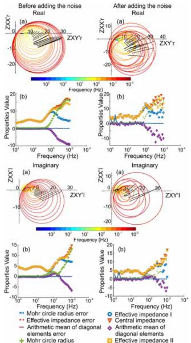
Figure 5. The response of the Mohr circle and its properties before adding the noise (left side) and after adding the noise (right side). The top figure is a real part response, and imaginary part results show the bottom figure.
