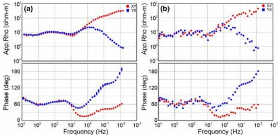
Figure 3. Resistivity and phase curves of RO station before adding synthetic noise (a) and after adding of synthetic noise (b).
