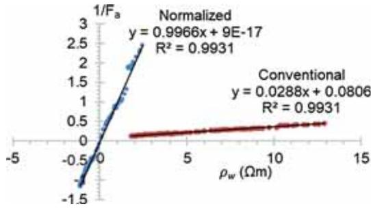
Figure 6. Models comparison between conventional and normalized resistivity data at Balik Pulau.
