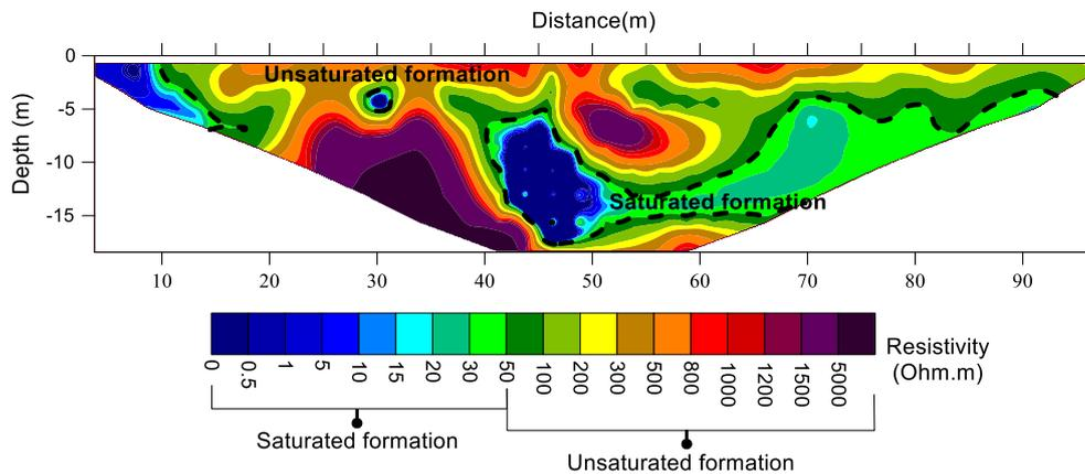
Figure 5. Resistivity profile at Teluk Kumbar that was separated into saturated and unsaturated medium.
