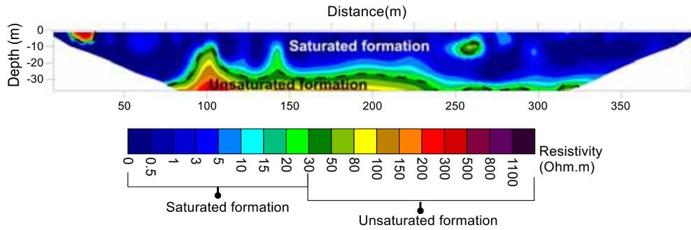
Figure 3. Resistivity profile at Balik Pulau that was separated into saturated and unsaturated mediums.
