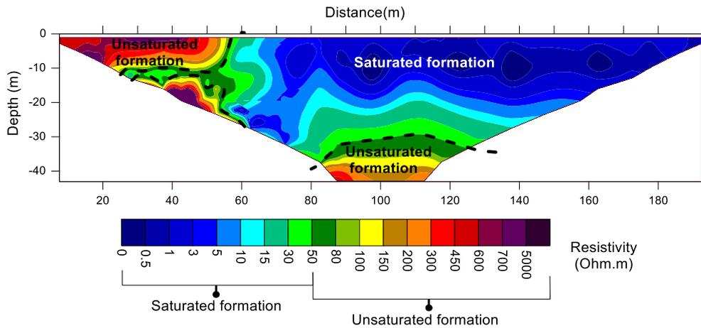
Figure 4. Resistivity profile at USM Minden that was separated into saturated and unsaturated mediums.
