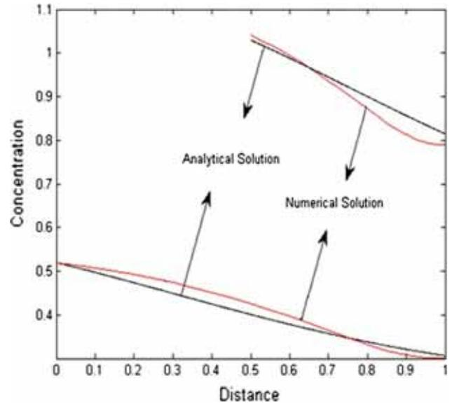
Figure 2. Contaminant concentration distribution with distance for sinusoidal velocity pattern.
