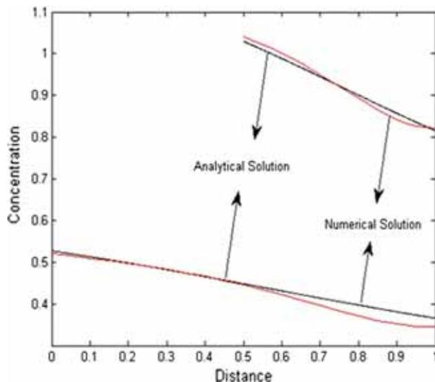
Figure 3. Contaminant concentration with distance for exponentially decreasing velocity.
