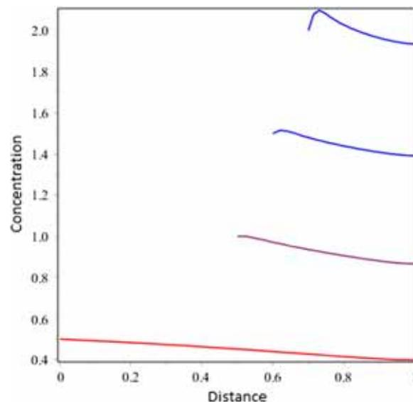
Figure 4. Contaminant concentration with distance for different sources acting one after another at  $x=0$ ,  $x=0.5$ ,  $x=0.6$  and  $x=0.7$  depicted, respectively, in (1), (2), (3) and (4).
