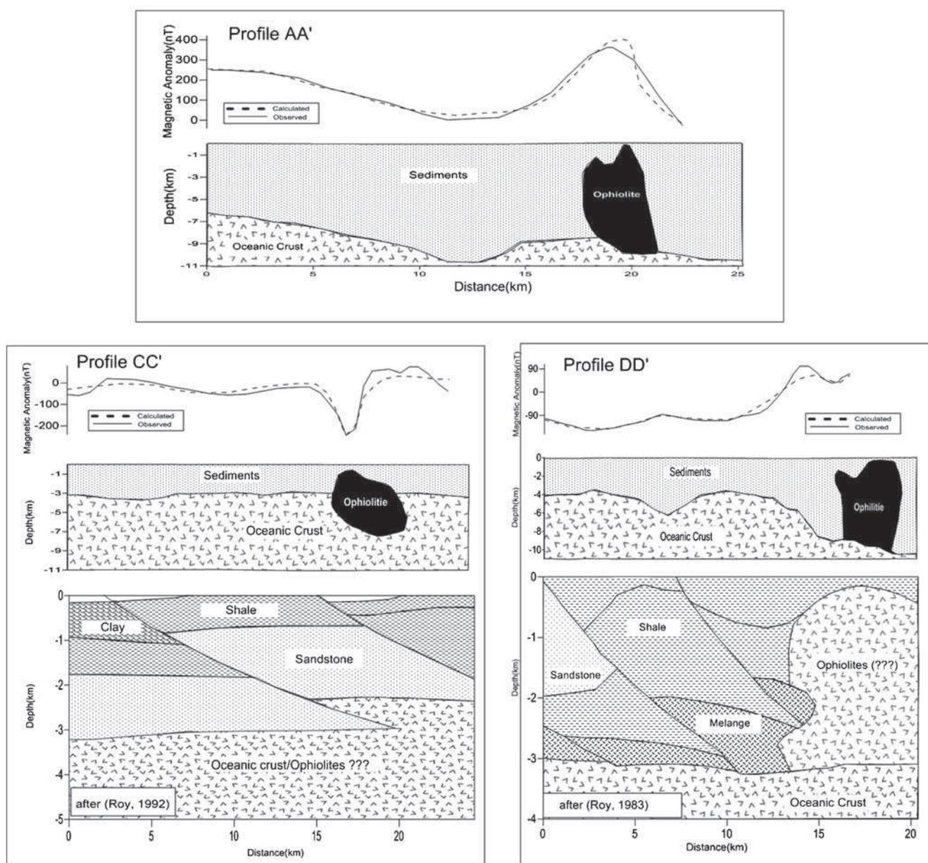
Figure 5. 2D modelling of magnetic anomalies along the profiles located in the north Andaman (profile AA'), middle Andaman (profile CC'), and south Andaman (profile DD') Islands region. The models reveal the presence of highly magnetized bodies related to ophiolites and ultramafic rocks along the east coast of Islands.
