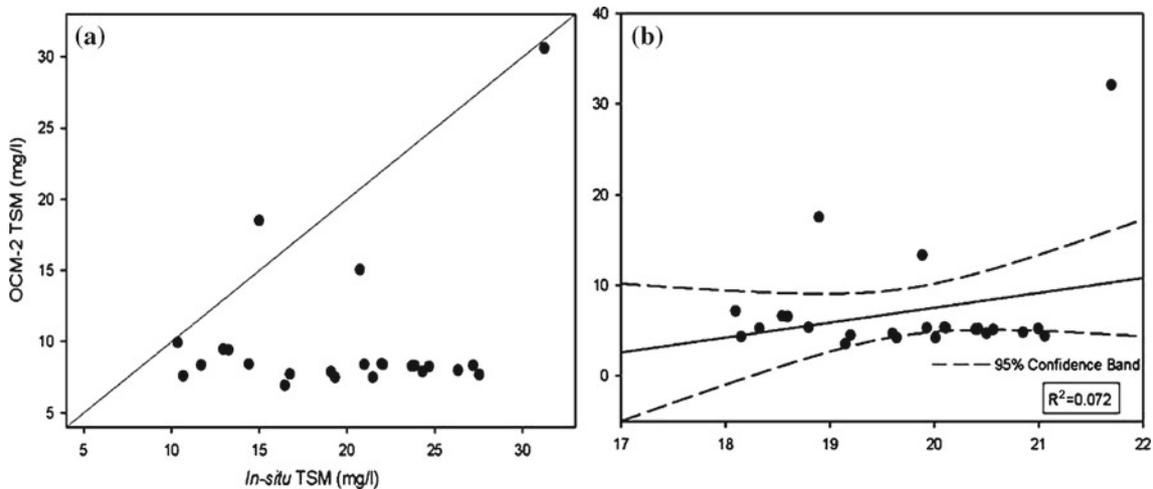
Figure 8. (a) Comparison and (b) regression plot of *in-situ* (moderate) vs. OCM-2 derived TSM.
