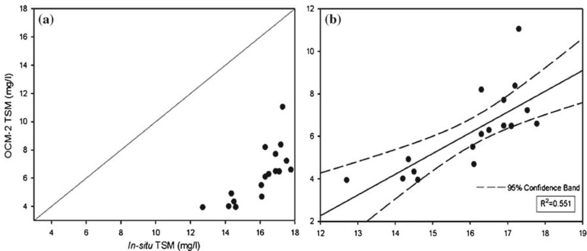
Figure 7. (a) Comparison and (b) regression plot of *in-situ* (low) vs. OCM-2 derived TSM.
