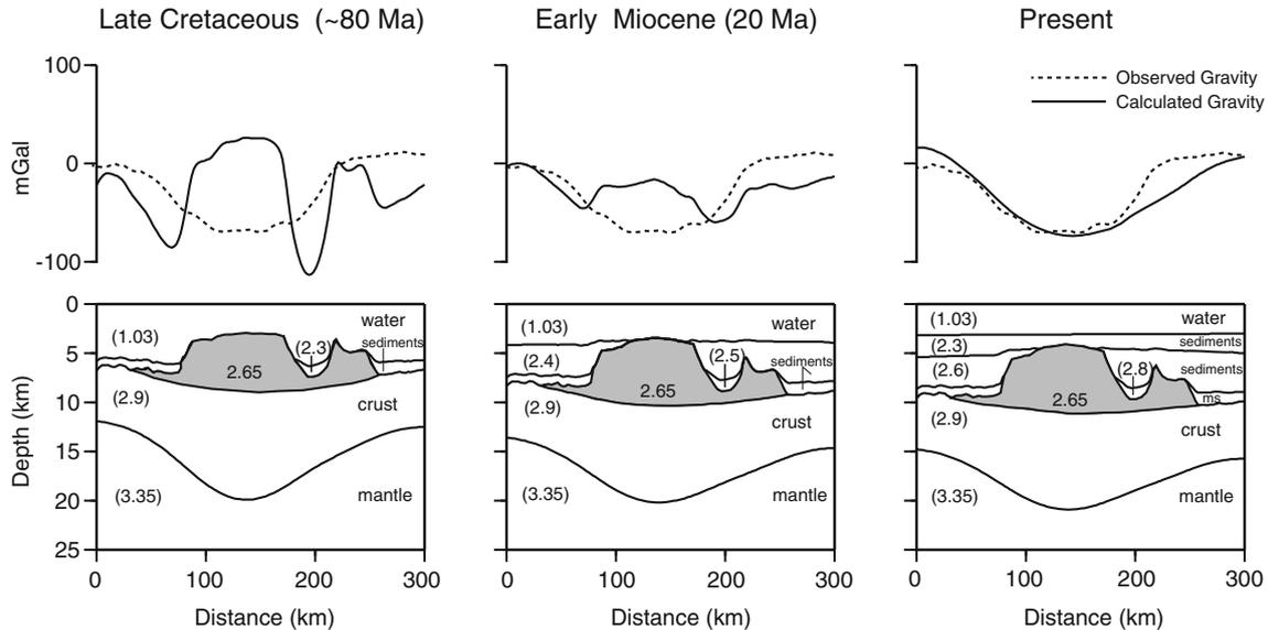
Figure 5. Reconstruction of the gravity anomalies over the 85°E Ridge through geological ages for the profile SK 107-07. The bottom panels represent the crustal structures for the respective periods. Note the change of gravity anomaly from positive to negative.
