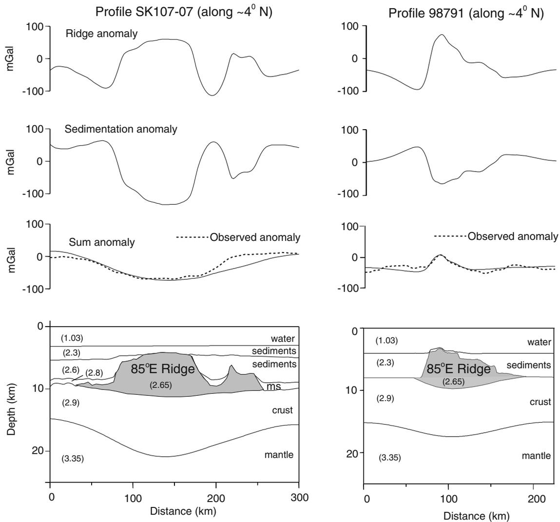
Figure 4. Crustal structure of 85°E Ridge along profile SK107-07 and 98971 along with different anomaly components (see details in text) obtained from process oriented gravity modelling. The values in bracket represent density for each layer in  $\text{g cm}^{-3}$ . The sum anomaly computed for best fitting  $T_e$  (10 km) is shown along with the observed gravity anomaly for both the profiles. ms indicates metasediments.
