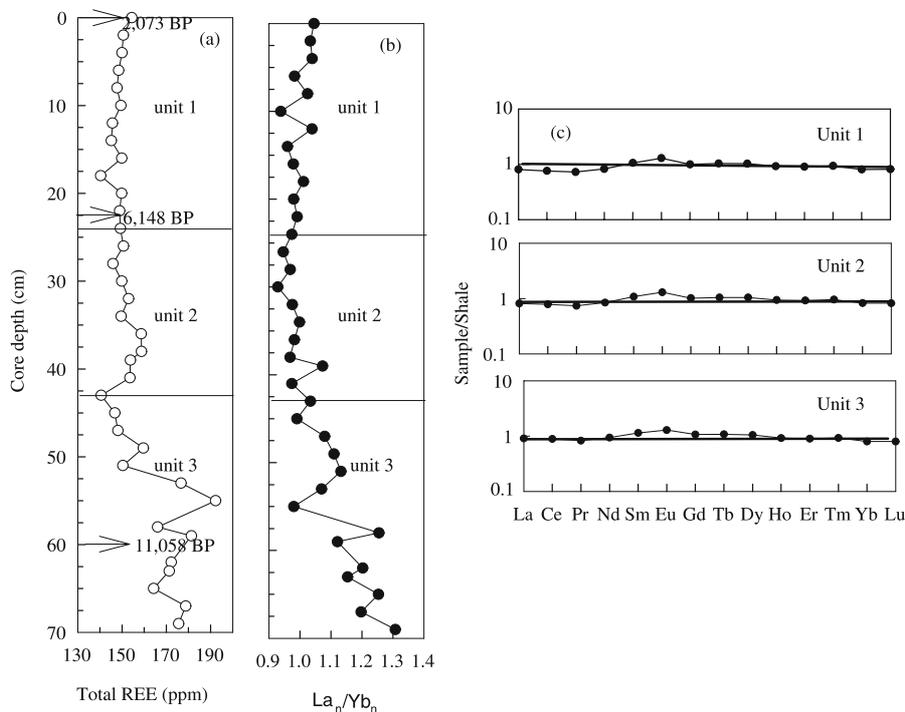
Figure 7. Down-core REE variations: (a) total REE, (b)  $La_n/Yb_n$ , and (c) shale normalized average REE patterns in three units. Observe a change in the  $La_n/Yb_n$  ratios between unit 3 and in units 2 and 1 suggesting a change in the provenance.
