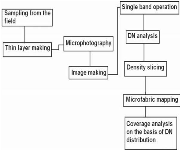
Figure 2. Flowchart of digital operation.
