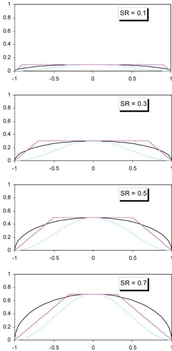
Figure 2. Comparison between cross sections of the semi-sine, trapezoidal and semi-elliptical hills. In the two first shape ratios, the trapezoidal and in the two last shape ratios, the semi-elliptical cross section has the largest area. In all of the cases, the semi-sine cross section has the smallest area.
