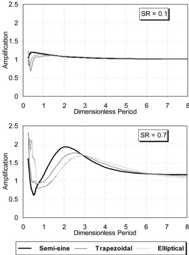
Figure 9. Incidence of a vertically propagating plane SV wave. Amplification curves at the crest of trapezoidal, semi-sine and semi-elliptical shaped hills, considering two limiting shape ratios of 0.1 and 0.7 and a Poisson ratio of 0.33.
