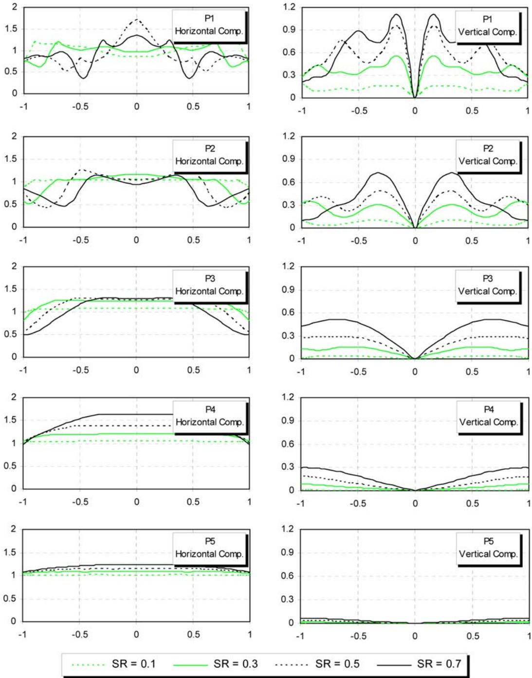
Figure 5. Incidence of a vertically propagating plane SV wave. The horizontal and vertical components of amplification curves for receivers between  $x = -b$  and  $x = b$  at surface of 2D trapezoidal shaped hills with different shape ratios and a Poisson ratio of 0.33. The amplification curves are categorized according to the wavelength of the incident wave.
