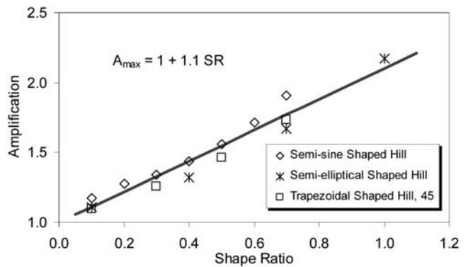
Figure 7. Incidence of a vertically propagating plane SV wave. The relation between maximum amplification factor at the crest of 2D semi-sine, semi-elliptical and trapezoidal shaped hills and shape ratio; averaged over the Poisson ratio range of 0.1 to 0.4.
