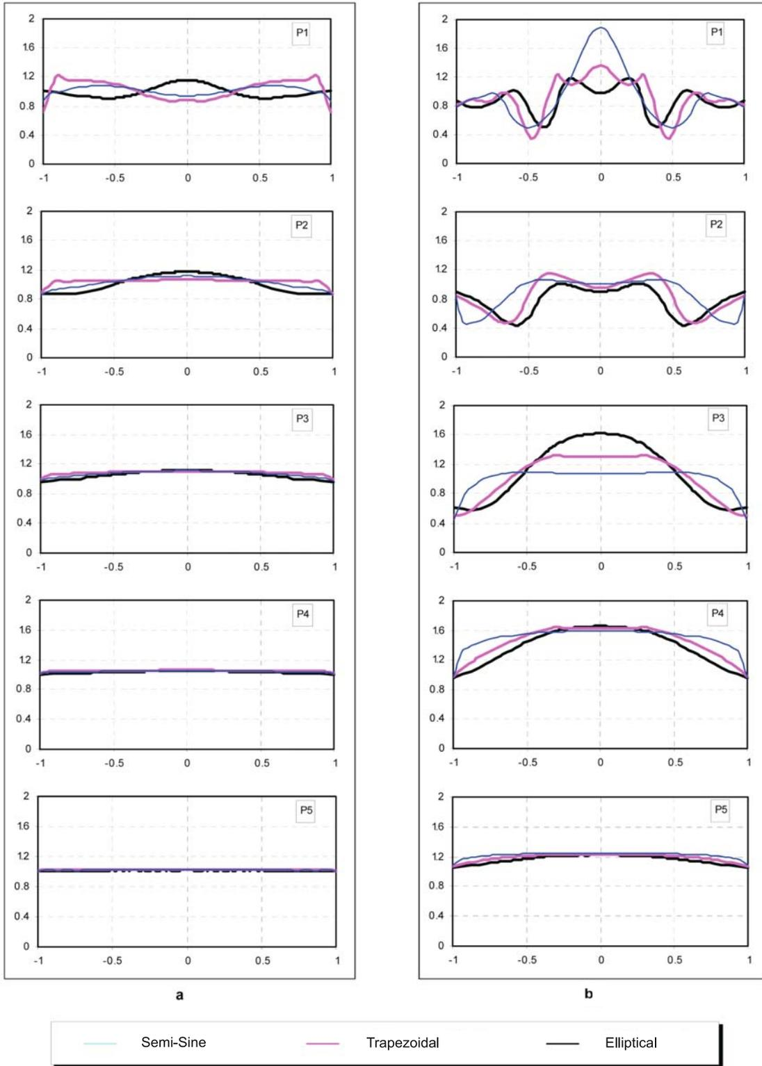
Figure 10. Incidence of a vertically propagating plane SV wave. Comparison of the shape effects on the amplification curves of the crest and rim of 2D semi-sine, semi-elliptical and trapezoidal shaped hills with a Poisson ratio of 0.33 and two limiting shape ratios of 0.1 and 0.7. The comparisons are made for five periodic sub-intervals.
