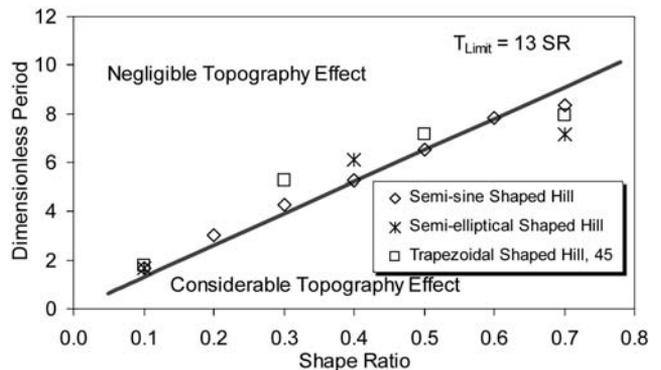
Figure 8. Incidence of a vertically propagating plane SV wave. The relation between limiting dimensionless period and shape ratio. In the areas above the line, the amplification effect of 2D hills could be practically ignored; that is, the amplification is equal or less than 1.1.
