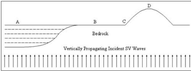
Figure 1. A schematic view of different site effect conditions subjected to the same incident waves. Points A, B, C and D respectively indicate, the ground surface of a soil stratum consisting of multiple layers with different mechanical properties overlying the bedrock, the outcrop of the rock on the flat half-plane, toe of the homogenous rocky hill and the crest of the hill.
