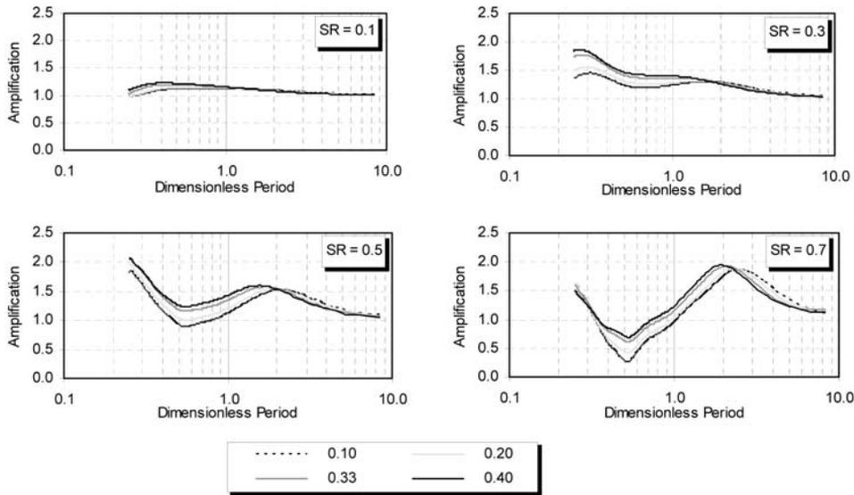
Figure 13. Incidence of a vertically propagating plane SV wave. Effect of Poisson ratio on the amplification curves of the crest of the semi-sine shaped hills versus different shape ratios. The vertical axis depicts the ratio of the cross section area of the hill to its square half width, while the horizontal axis shows the shape ratio.
