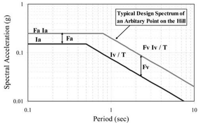
Figure 14. Schematic design spectrum of 2D rocky hills in terms of short period ( $I_a$ ) and long period ( $I_v$ ) seismic hazard levels as well as short period ( $F_a$ ) and long period ( $F_v$ ) spectral amplification factors.
