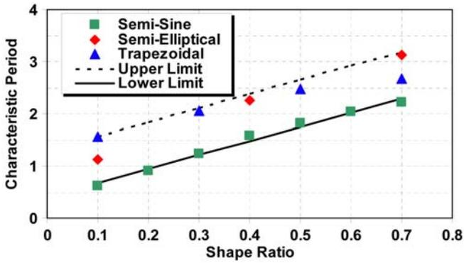
Figure 11. Characteristic periods of the semi-sine, semi-elliptical and trapezoidal shaped hills *versus* shape ratio (solid points). Two straight lines also indicate the upper and lower limits of characteristic periods for the hills. The characteristic periods are estimated for the incidence of a vertically propagating plane SV wave and for the hills with a Poisson ratio of 0.33.
