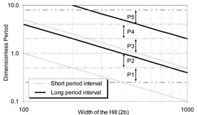
Figure 15. Dimensionless period bands (P1 to P5) encountered in averaging the spectral amplification over the short period (0.1 to 0.5 s) and long period (0.4 to 2.0 s) intervals, assuming shear wave velocity of 1000 m/s.
