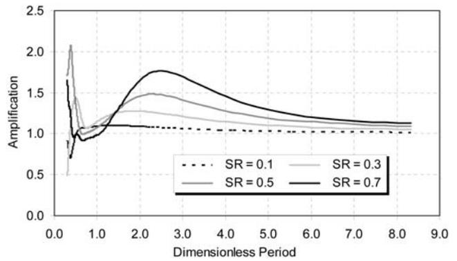
Figure 6. Incidence of a vertically propagating plane SV wave. Amplification curves of the crest of 2D trapezoidal hills with a Poisson ratio of 0.33 *versus* shape ratio.
