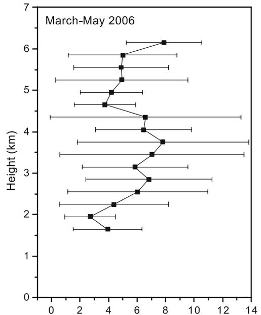
(b) Vertical Gradient of Horizontal Wind ( $\times 10^{-3} \text{ s}^{-1}$ )
