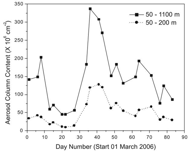
Figure 8. Day-to-day variation of lidar-derived aerosol column content in the 50–200 m and 50–1100 m levels during the period 1 March–22 May 2006.
