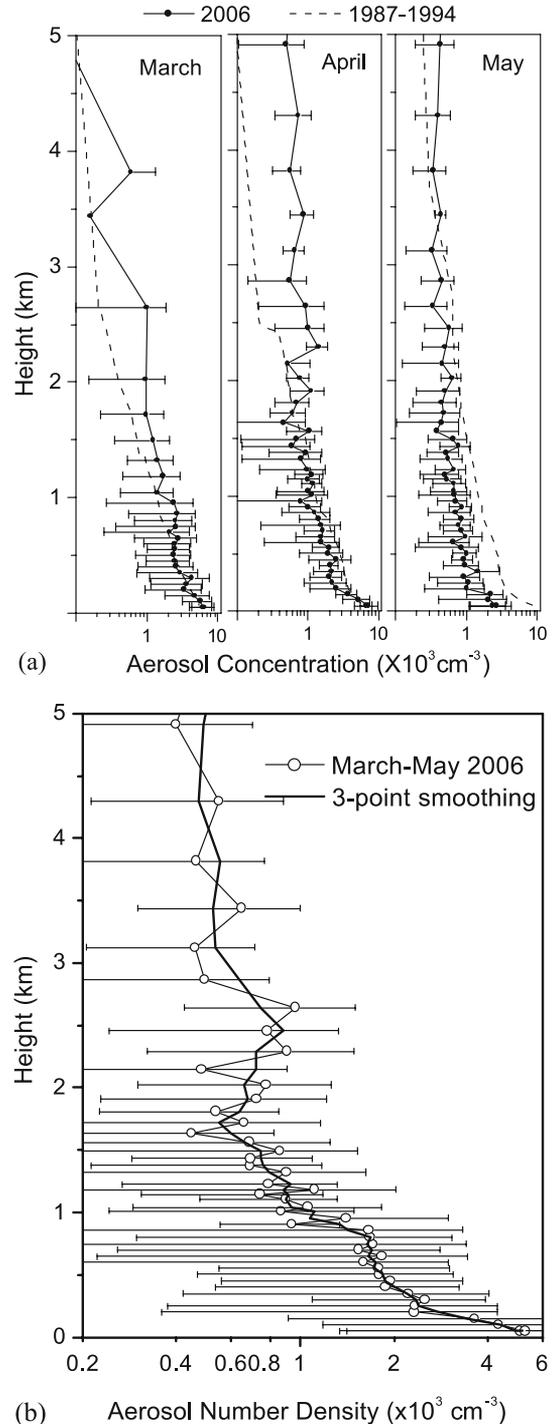
Figure 2. (a) Monthly mean vertical distribution of aerosol number density for March, April and May 2006 along with corresponding month's mean for the period 1987–1994 (horizontal bars at each height indicate standard deviation). (b) Mean vertical distribution of aerosol number density for the period 1 March–22 May 2006 (horizontal bars at each height indicate standard deviation and thick solid line indicates 3-point smoothing).
