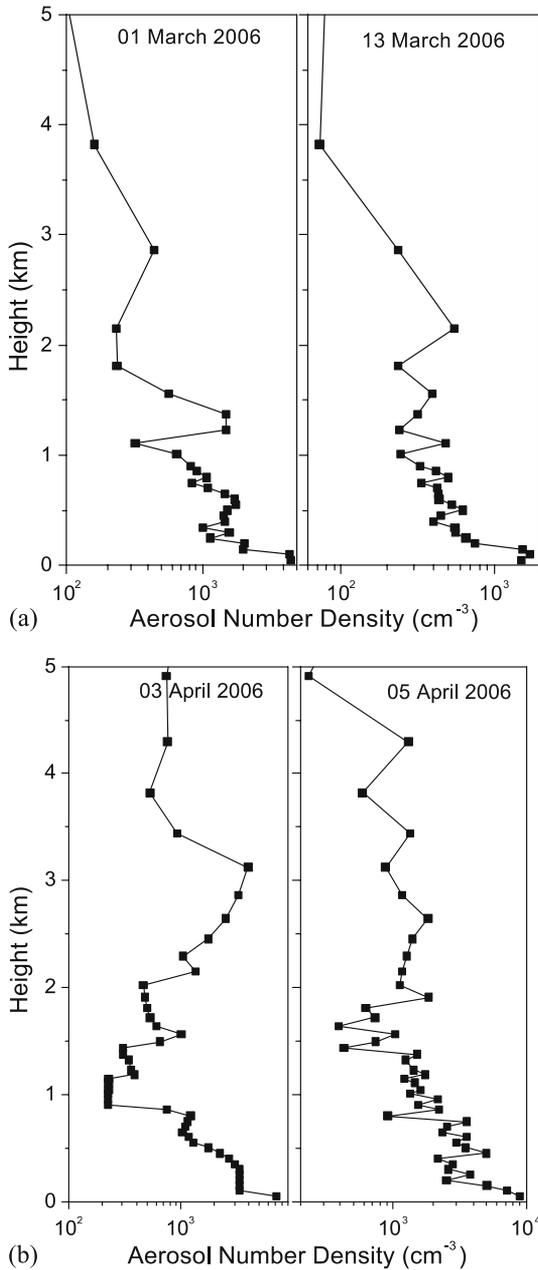
Figure 1. Lidar-derived vertical profiles of aerosol number density on two typical days (a) 1 and 13 in March 2006, and (b) 3 and 5 in April 2006.
