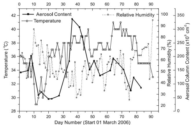
Figure 9. Day-to-day variation of aerosol column content in the 50–1100 m level, surface maximum temperature and relative humidity for the period 1 March–31 May 2006.
