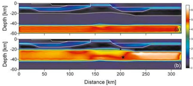
Figure 5. Computed maximum shear stresses in MPa for the case of prescribed horizontal displacement at the right boundary to simulate plate tectonic stresses. (a) elastically weak lower crust on strong upper mantle, and (b) strong lower crust and weak upper mantle.
