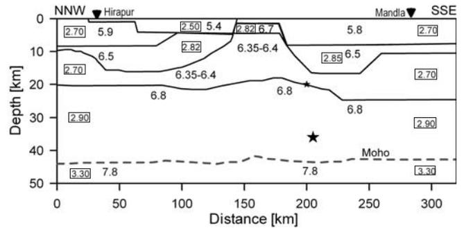
Figure 2. Simplified crustal structure along the Hirapur–Mandla profile (profile P-I in figure 1) obtained by integrated deep crustal seismic and gravity data (after Murty *et al* 2004). Values in large fonts are  $P$ -wave velocities in km/s and those enclosed in boxes are density in  $\text{gm/cm}^3$ .
