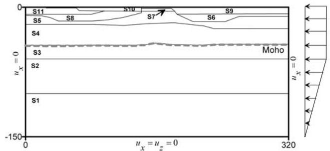
Figure 3. Geometry of the model used for finite element discretization along with boundary conditions at left, right, and bottom boundaries. Also shown is prescribed horizontal displacement boundary condition at the right boundary for the case discussed in section 5.2. The finite element model has been constructed from 11 patches marked as S1–S11. Material parameters of these patches are given in table 1.
