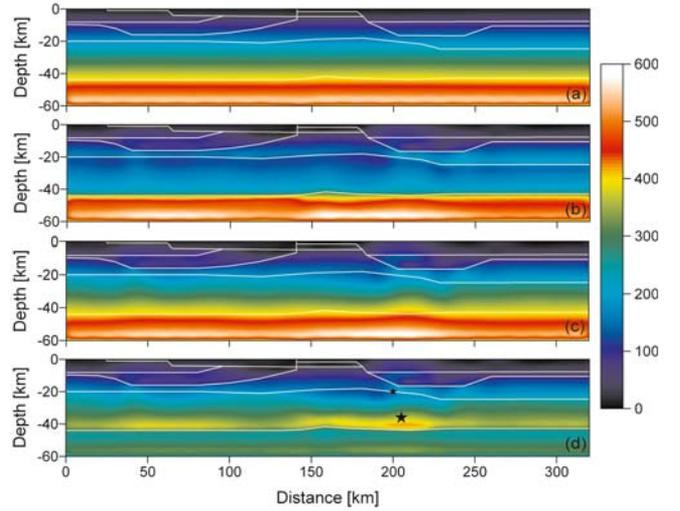
Figure 4. Computed maximum shear stresses in MPa for various model cases: (a) only density heterogeneities, (b) both density and mechanical property variations for elastically weak lower crust and strong upper mantle, (c) same as (b) but with elastically strong lower crust, and (d) strong lower crust and weak upper mantle. Large star represents the focal depth of the 1997 Jabalpur earthquake and small star corresponds to the 2001 Jabalpur earthquake.
