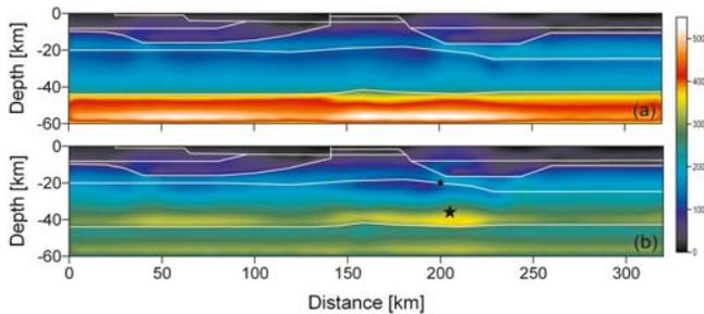
Figure 6. Maximum shear stresses in MPa after combining gravity stress shown in figure 4 and tectonic stress shown in figure 5 for the cases (a) weak lower crust, and (b) strong lower crust and weak upper mantle.
