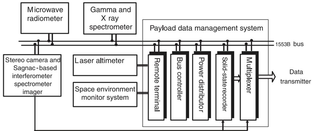
Figure 1. Payloads and data management scheme for the Chang'E-1 mission.
