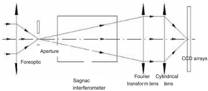
Figure 3. Schematic of the spectrometer imager.
