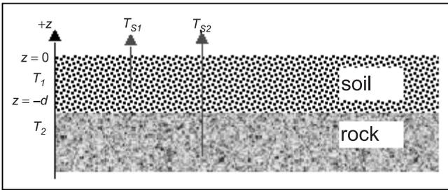
Figure 8. Schematic showing the emission of the microwave brightness temperature radiation from the lunar surface.
