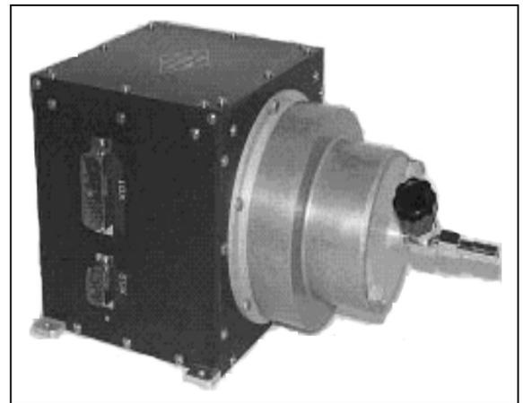
Figure 11. Solar wind detector.
