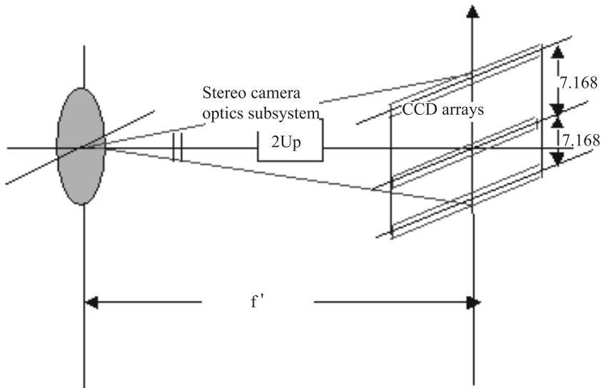
Figure 2. Schematic diagram of Chang'E-1 stereo camera.
