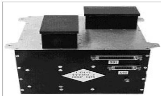
Figure 7. Chang'E's X-ray spectrometer.
