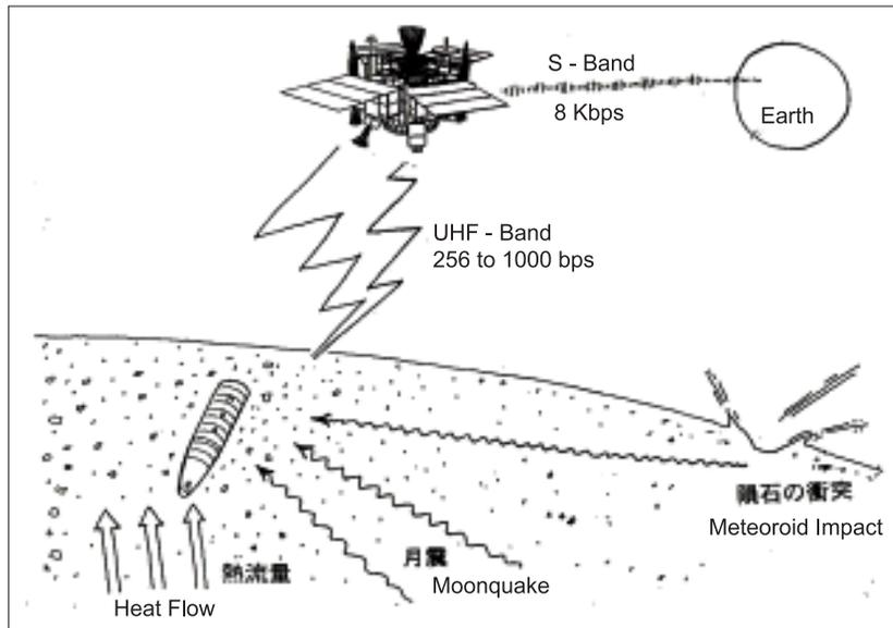
Figure 1. Schematic diagram of the Lunar-A penetrator operation.
