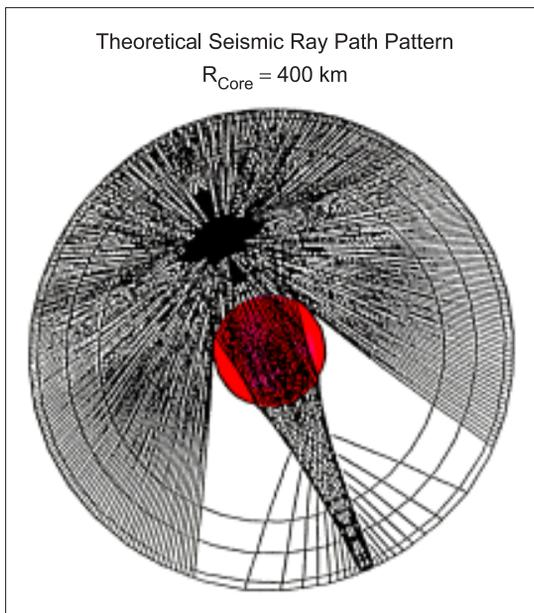
Figure 2. Theoretical seismic ray paths from a deep moonquake located at a depth of 900 km. The strong ray focusing is observed at an antipodal site of the epicenter.
