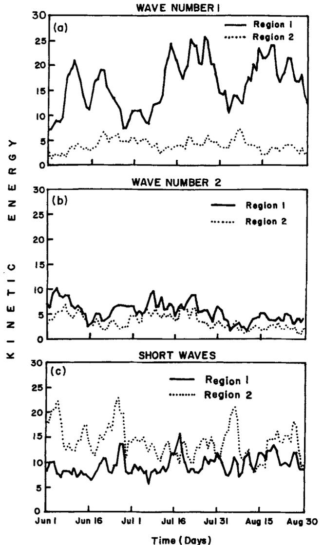
Figure 3. Temporal variations of kinetic energy (unit:  $m^2 s^{-2}$ ) of (a) wavenumber 1, (b) wavenumber 2 and (c) wavenumbers 3 to 10 over Region 1 (equator to 20°N) and Region 2 (20°N to 40°N) at 850 hPa for the period from 1st June to 31 August 1991).
