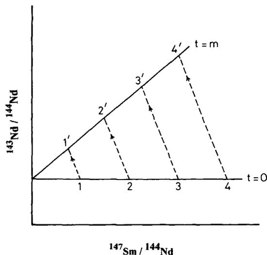
Figure 1. Sm-Nd isochron diagram. Numbers 1, 2 etc. represent rock samples which have variable Sm/Nd ratios but with one value of initial Nd isotopic ratio at time ' $t$ ' before present. Numbers 1', 2' etc. represent the present positions of the same rock samples, as measured today.
