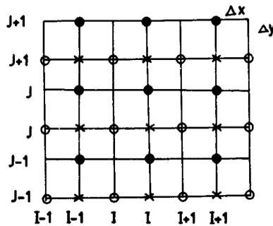
Figure 2. Staggered grid finite difference mesh used in the discretization of governing equations. Points marked ●, ○ and × are  $u$ ,  $v$  and  $\eta$  points respectively.
