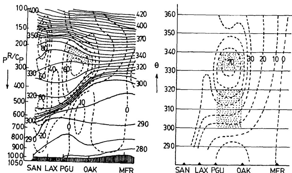
Figure 1. A comparison of cross-section through a front in isobaric (a) and isentropic (b) coordinates. (Bleck and Shapiro 1976; and Shapiro and Hastings 1973).
