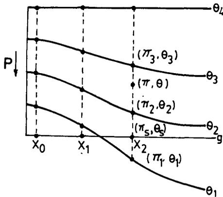
**Figure 2.** Illustration of the vertical extrapolation technique for permitting the evaluation of the finite-difference approximations near the intersection of isentropic coordinate surface,  $\theta_1$ , with the earth's surface  $g$  (Shapiro 1975).
