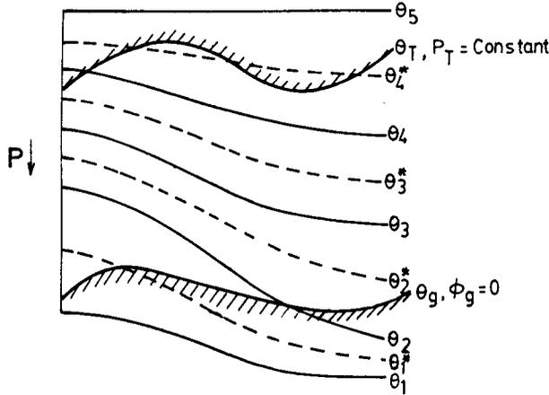
**Figure 3.** Vertical discretization scheme in our model.  $\theta_g$ , the rigid surface with constant height and  $\theta_T$ , the free surface of constant pressure of the physical domain. This physical domain is defined inside the computational domain ( $\theta_1 - \theta_5$ ).
