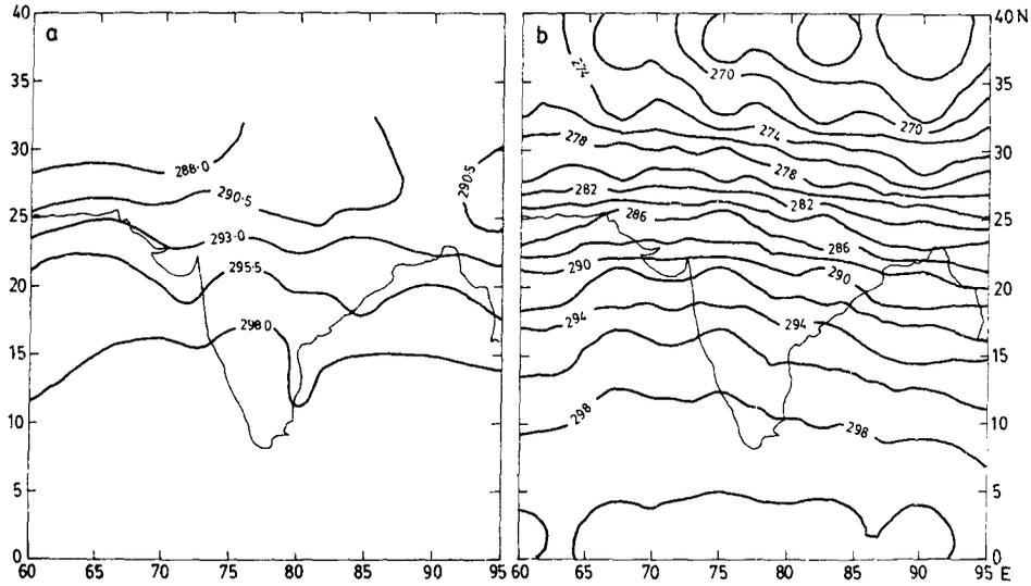
**Figure 1.** Observed (a) and model-simulated (b) surface air temperature distributions (K) for winter over the Indian sub-continent.
