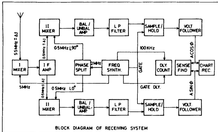
Figure 2. Block diagram of the phase coherent receiving system.
