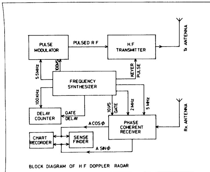
Figure 1. Block diagram of the HF doppler system.
