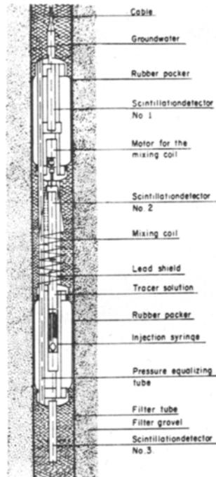
**Figure 3.** Borehole probe for determination of filtration velocity of groundwater.
